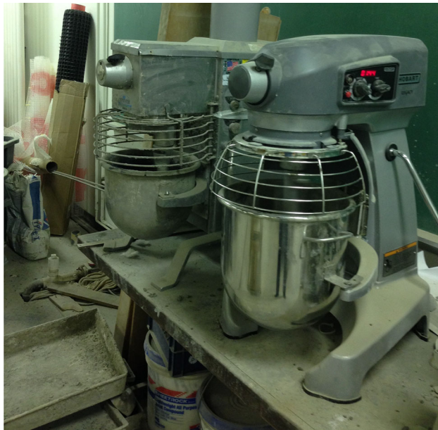
Fig. 2 Two mechanical mixers used to prepare LMM mixes.
