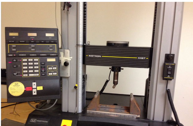
Fig. 3 Three-point bending test setup.
