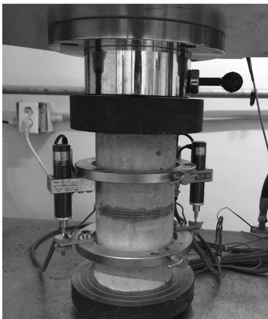
Fig. 4 Test setup for cylindrical specimens.
