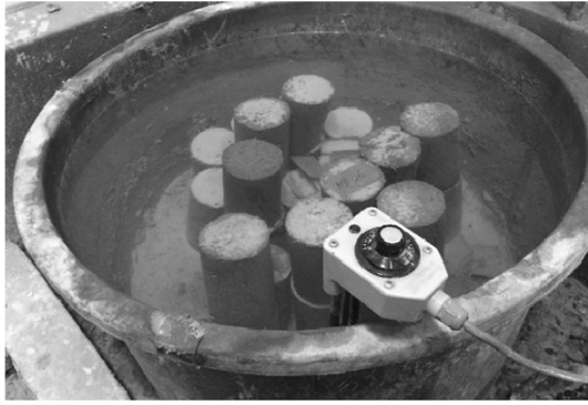
Fig. 3 Curing specimens following ASTM C31.
