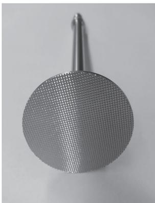
**Fig. 1** Serrated bob plate used in the measurements to minimize the effects of slip and settling.
