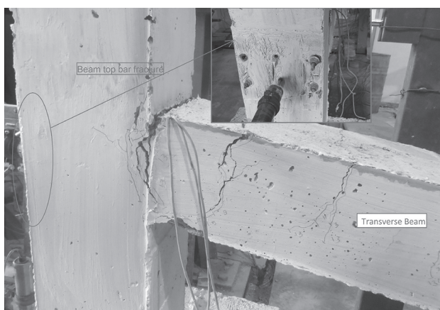
Fig. 6 Fracture of top bars at the end of the test.
