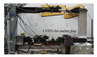
Fig. 6 Test setup for shear tests of cast-in anchors in plastic hinge zone.
