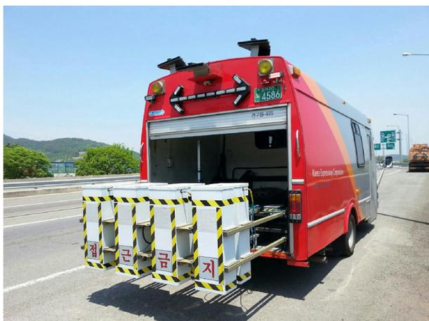
Fig. 1 Air-coupled GPR system used for concrete bridge deck survey.
