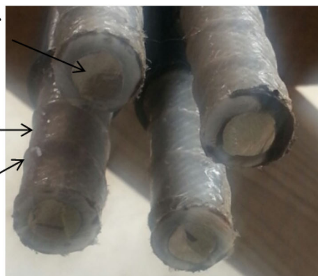
Fig. 1 Geometry and product of GFRP and deformed steel hybrid bar.
