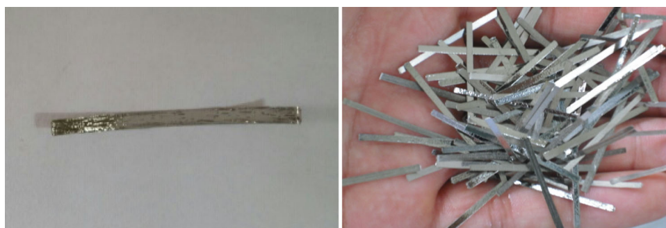
Fig. 1 Photos of amorphous micro steel fibres.
