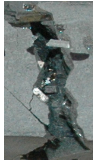
Fig. 10 Fracture of fibres in tensile failure of AMS fibre cementitious composite.
