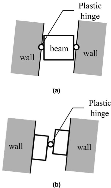
Fig. 13 Plastic behavior that corresponds to formation of plastic hinges. a Formation of plastic hinge at wall-beam joints, b Formation of plastic hinge at beam center.
