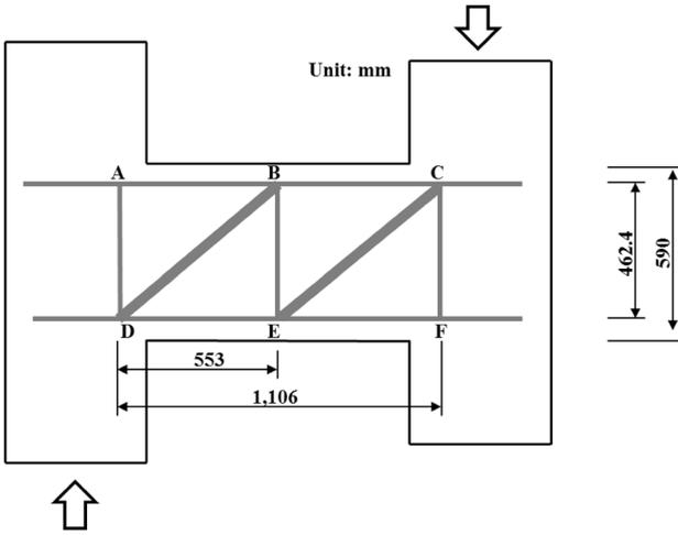
Fig. 6 Truss model for short coupling beam.
