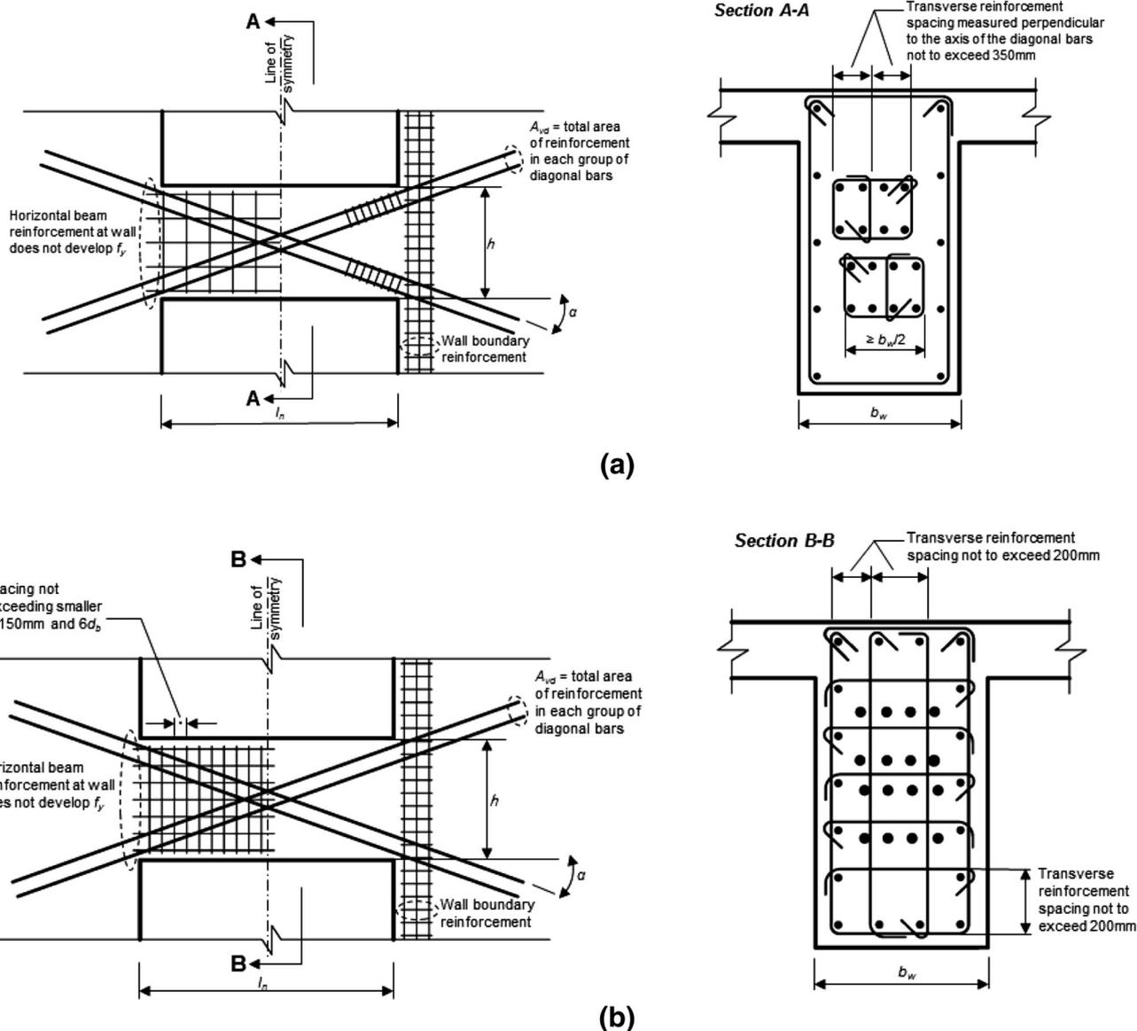
Fig. 3 Reinforcement details for short coupling beam in ACI 318 (2011). a Confining diagonal bars, b Confining beam.
