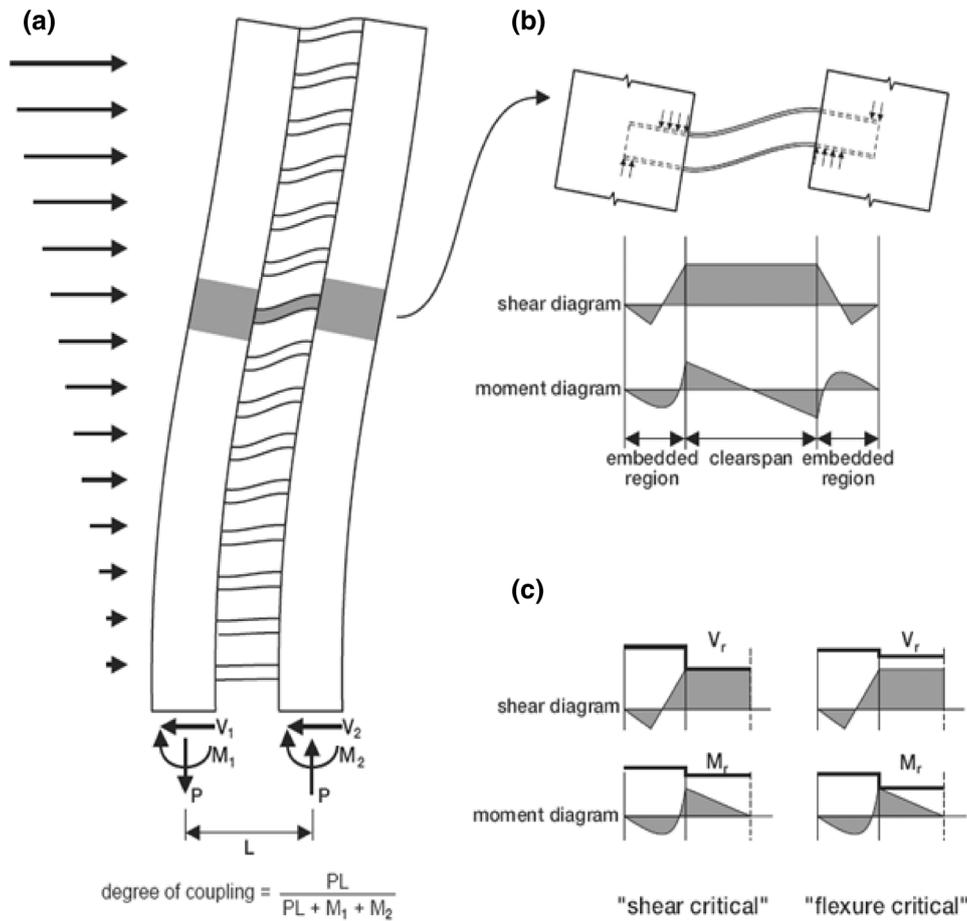
Fig. 1 Structural behavior of coupling beam.
