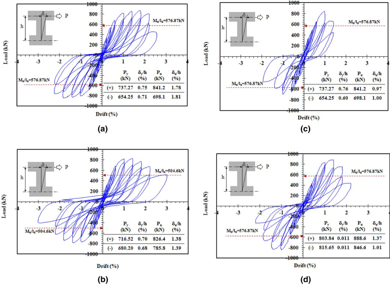
Fig. 11 Load–drift curves of specimens. a B-1-H, b B-1-HA, c B-2, d B-2-H.
