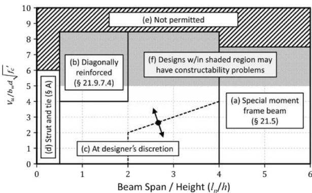
Fig. 2 Design concept for coupling beam in ACI 318 (2011).
