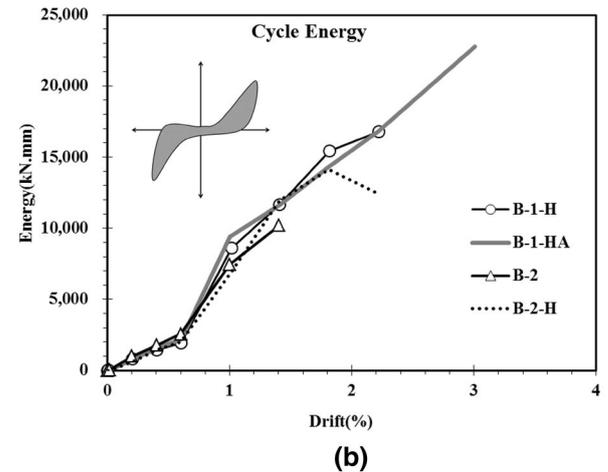
Fig. 14 Comparison of dissipated energy values: a accumulated energy, b cyclic energy.
