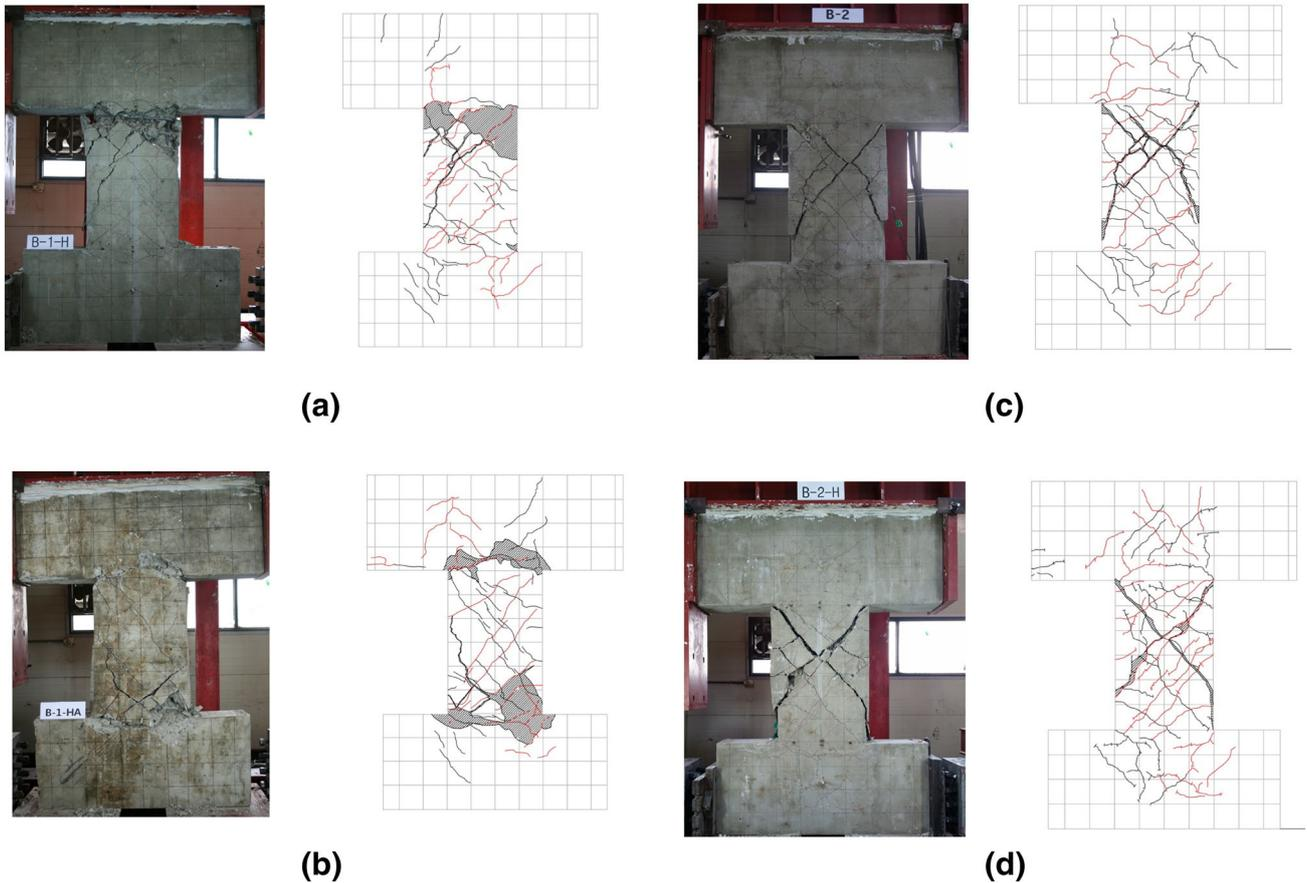
**Fig. 10** Failure patterns of specimens. a B-1-H, b B-1-HA, c B-2, d B-2-H.
