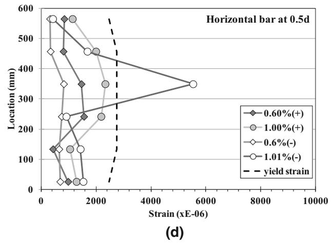
Fig. 15 Strain levels of horizontal bars. a B-1-H, b B-1-HA, c B-2, d B-2-H.
