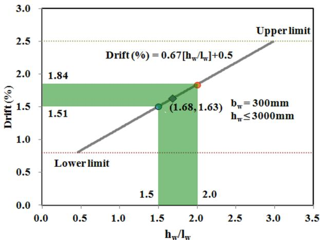
Fig. 4 Drift of wall in wall-slab structure.
