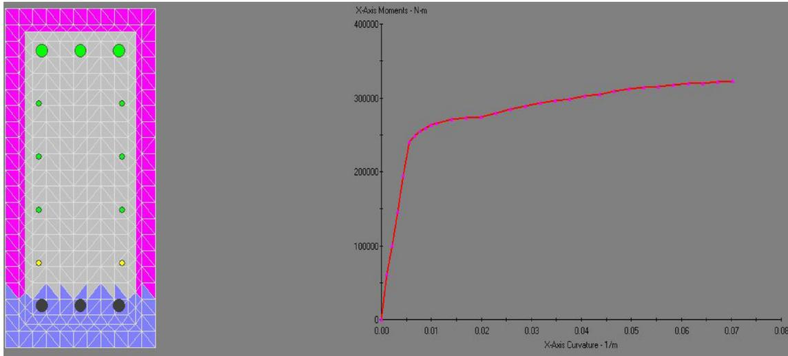
(2) When stirrup (2-(HD13+HD10)@100) reaches its yield strength due to shear force,
