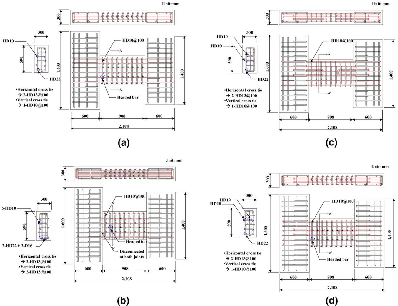
Fig. 5 Specimen configurations and reinforcement details. a B-1-H, b B-1-HA, c B-2, d B-2-H.
