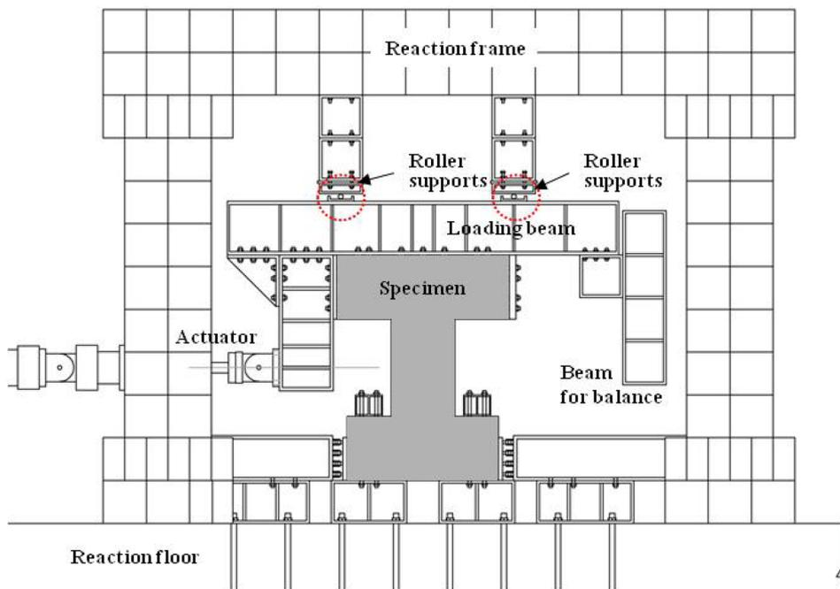
Fig. 7 Test setup for short coupling beams.
