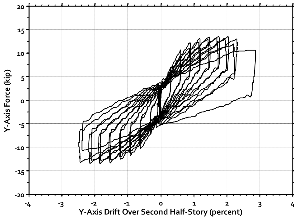
Figure C-8: Specimen B2 – Load versus Second Half-Story Drift in Y-Direction
