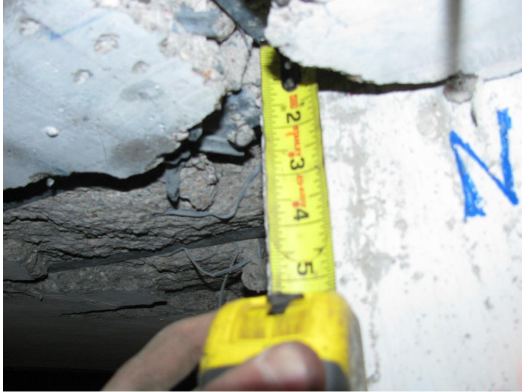
Figure 3-12: Specimen B1 – Bottom View of North-East Corner of Slab-Column Connection After Test
