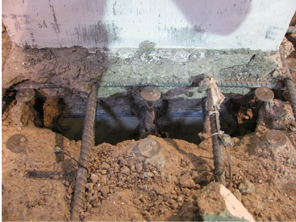
Figure 3-16: Specimen B2 – Connection Region where Severely Degraded Concrete was Removed by Hand After Test
