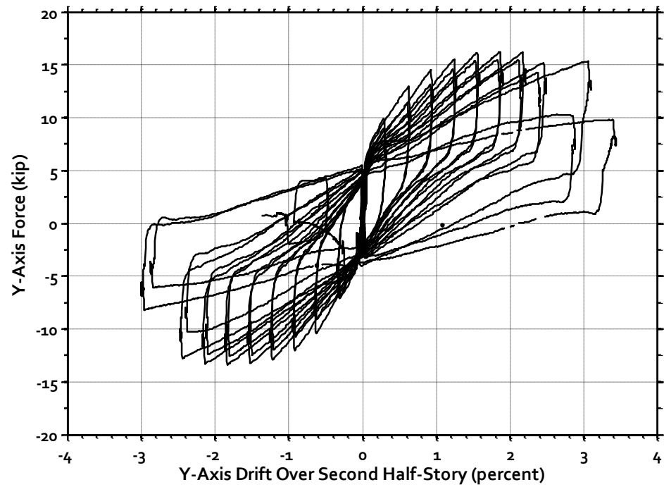
Figure C-12: Specimen B3 – Load versus Second Half-Story Drift in Y-Direction
