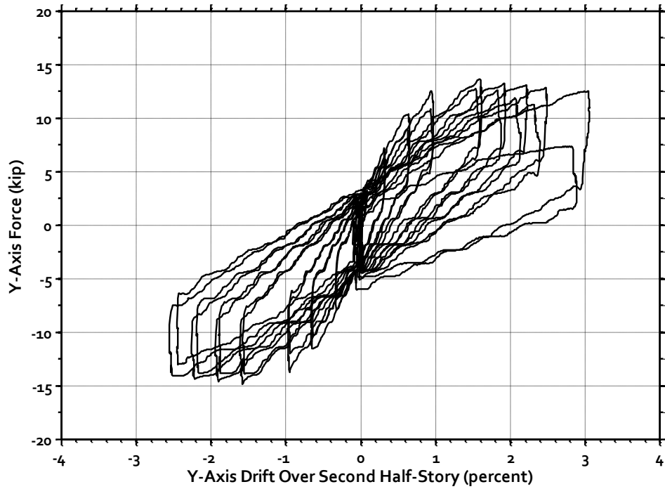
Figure C-4: Specimen B1 – Load versus Second Half-Story Drift in Y-Direction
