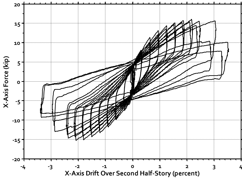
Figure C-14: Specimen B4 – Load versus Second Half-Story Drift in X-Direction
