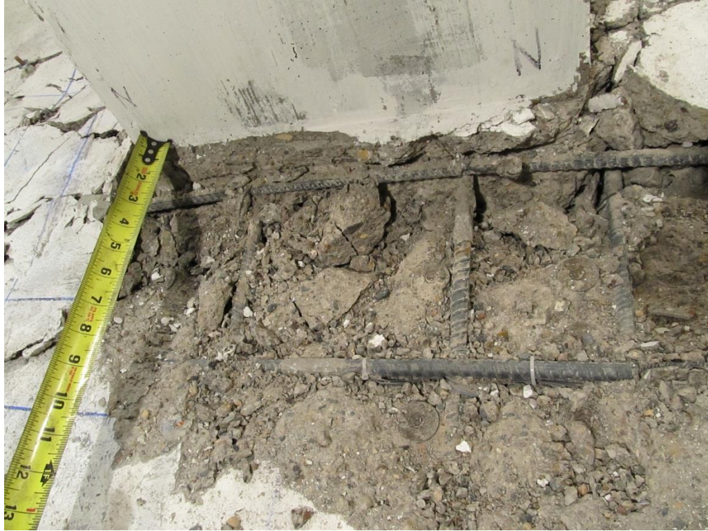
Figure 3-20: Specimen B4 – Gravel-Like Concrete within Connection Region
