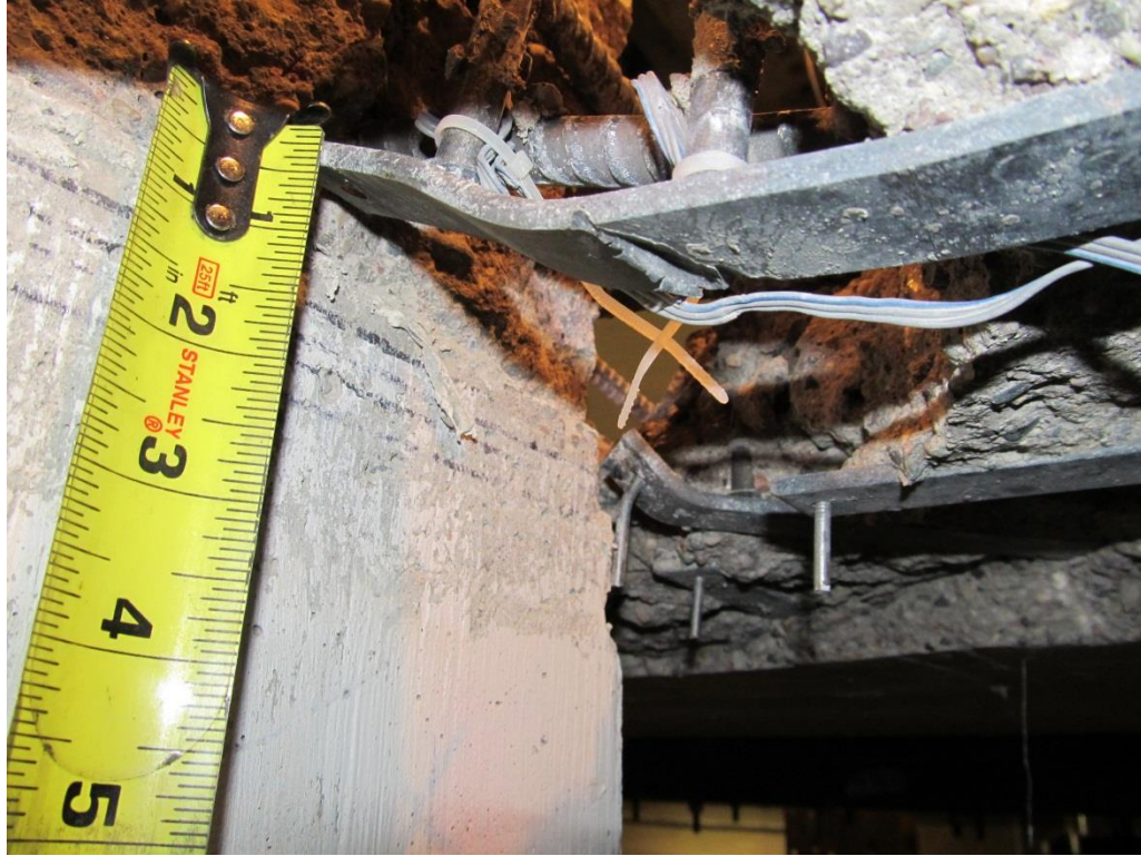
Figure 3-22: Specimen B4 – Bending of Base Rail on South-East Face of Column After Test
