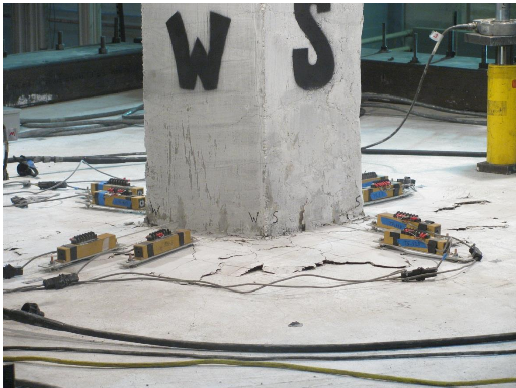
Figure 3-8: Specimen B3 – Connection Damage at 2.30% Drift, Point 1-2
