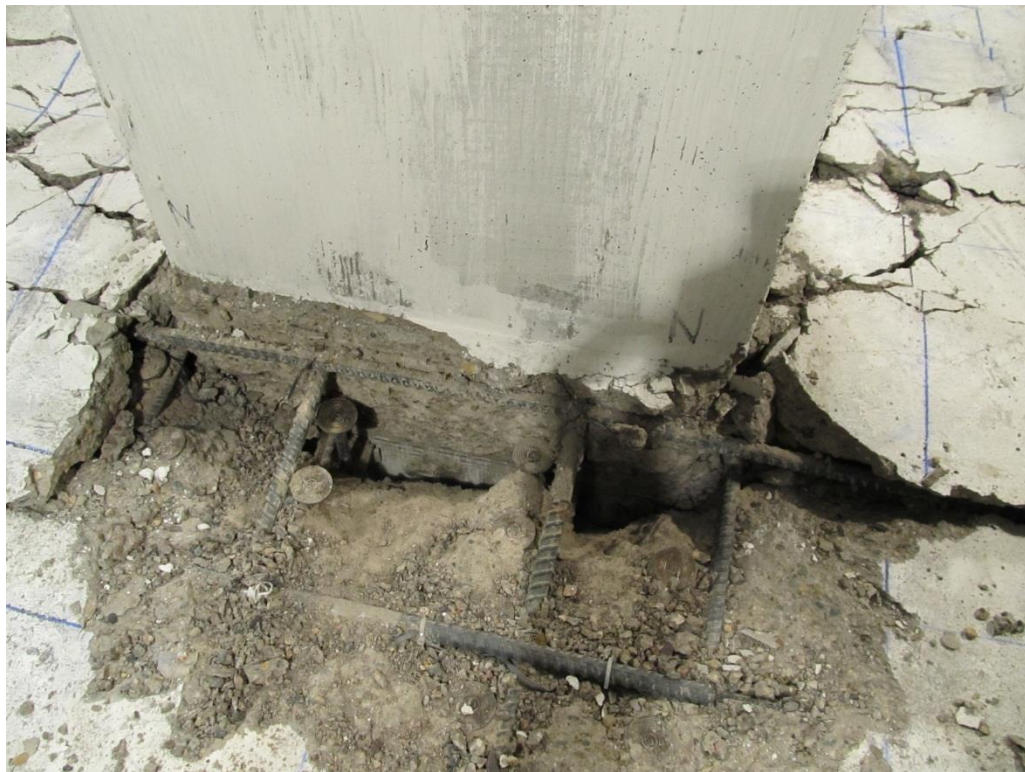
Figure 3-21: Specimen B4 – Void in Connection Region after Loose Concrete was Removed After Test
