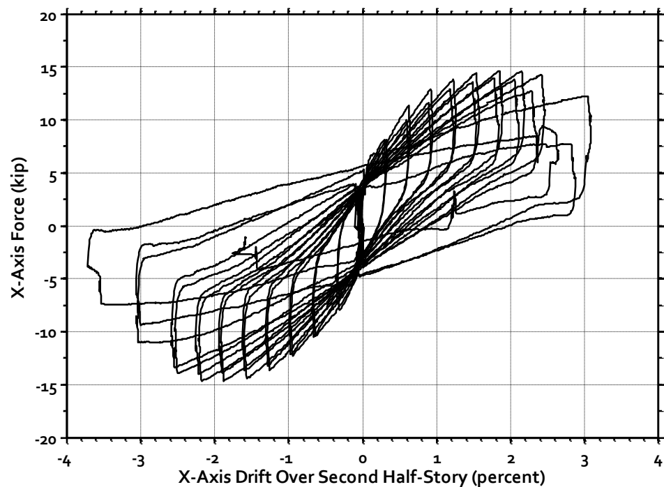
Figure C-10: Specimen B3 – Load versus Second Half-Story Drift in X-Direction
