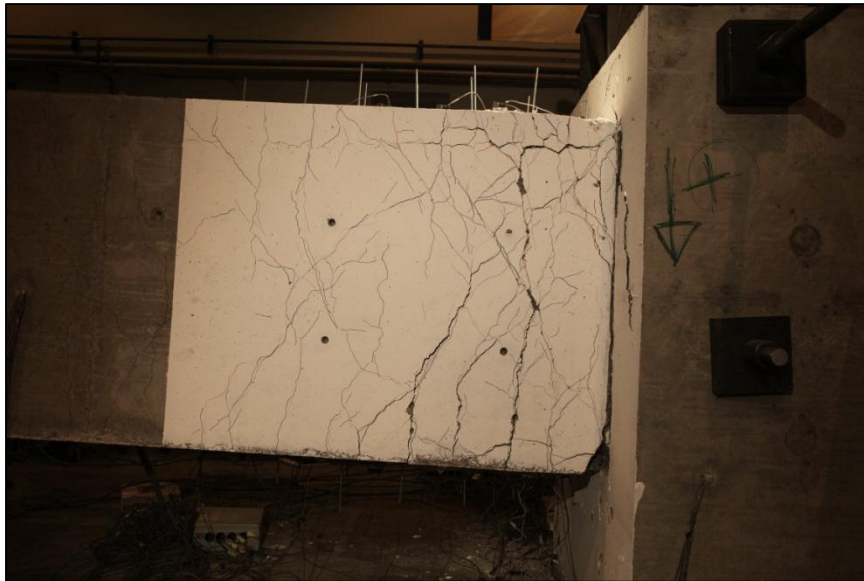
Figure 22 Beam 2: damage state during the second cycle with a peak drift ratio of 2.9% (instantaneous drift ratio = -2.9%).
