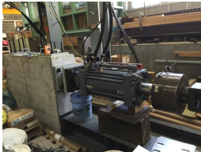
Figure 2.13: Hydraulic Actuator Connected to Concrete Reaction Block
