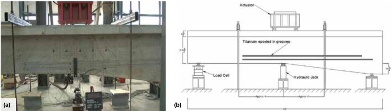
**Fig. 3:** Full-scale beam testing was used to verify the adequacy of the proposed repairs for the Mosier bridge: (a) photo of a strengthened beam prior to testing; and (b) schematic of test apparatus (Note: 1 ft = 0.30 m; 1 in. = 25 mm) (photo and schematic courtesy of Christopher Higgins, OSU)
