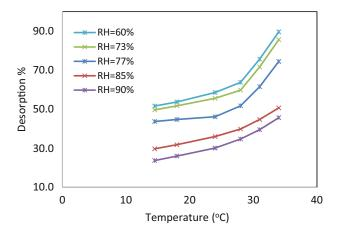
Fig. 3 Effect of temperature on desorption rate of MCA.
