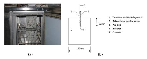
Fig. 10 Internal RH measurement a experimental diagram b schematic diagram.
