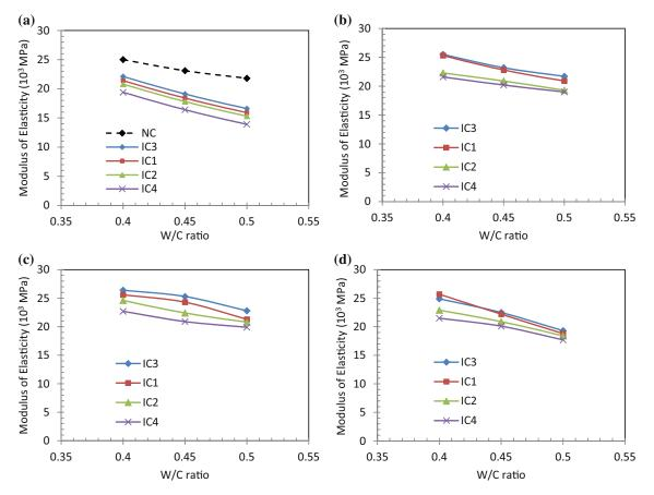
Fig. 7 Effect of w/c ratio on modulus of elasticity of samples a control samples with 0% replacement b IC samples with 10% replacement c IC samples with 20% replacement d IC samples with 30% replacement.
