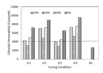
Fig. 9 Chloride permeability of samples for different curing conditions and different percent replacement at a constant w/c ratio of 0.4.
