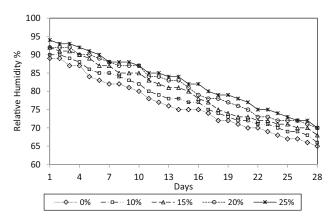
Fig. 11 Internal RH data of control samples and internally cured samples with respect to days.
