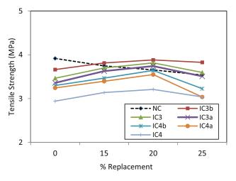
Fig. 13 Effect of percent replacement on splitting tensile strength (Phase II).
