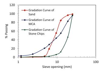
Fig. 2 Gradation *curves* of sand, masonry chip aggregate (MCA) and stone chips.
