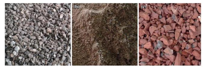
Fig. 1 Aggregates (a) stone chips (b) sand (c) masonry chip aggregate (MCA).
