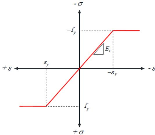
Fig. 15 Stress-strain curve for steel reinforcement.
