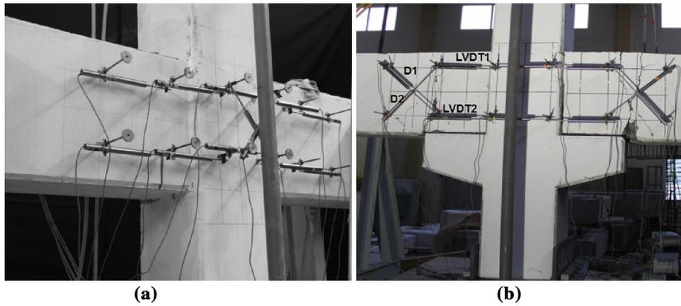
Fig. 12 Installation of LVDTs for a MONO, SP1-R, SP3 and b SP1, SP2, and SP3-R specimens.
