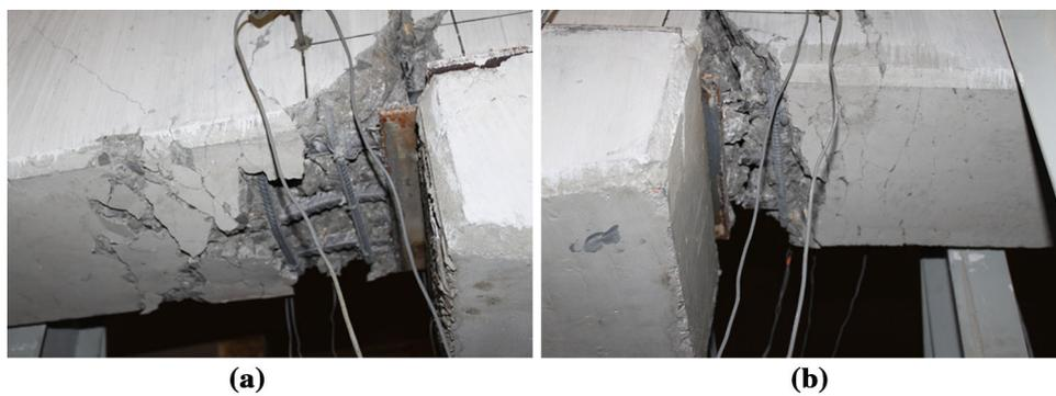
**Fig. 15** **a** Initiation of rebar buckling at the left beam (Beam 1) and **b** the rupture of rebars at the right beam (Beam 2) for SP1 specimen at 2.2% top drift.
