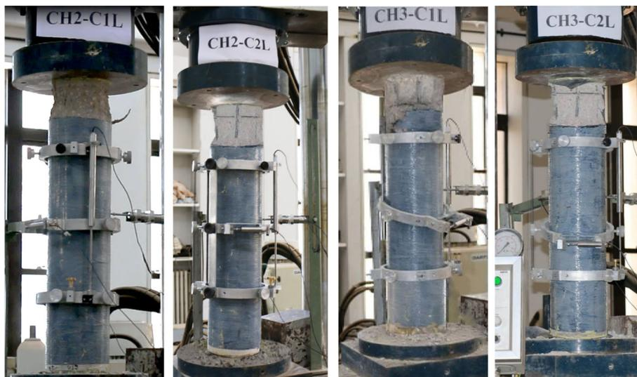
Fig. 7 Failure modes for CFRP wrapped specimens.
