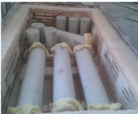
**Fig. 2** Sample arrangement of test specimens in electric furnace.
