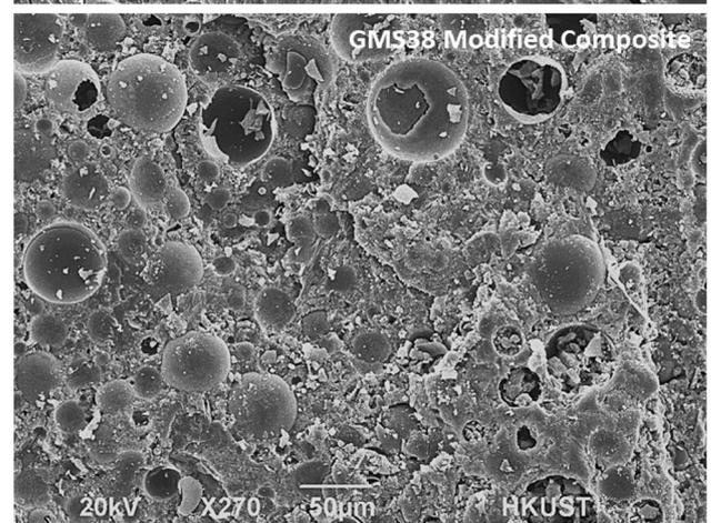
**Fig. 13** SEM images of fractured surfaces of composites containing LWFs.
