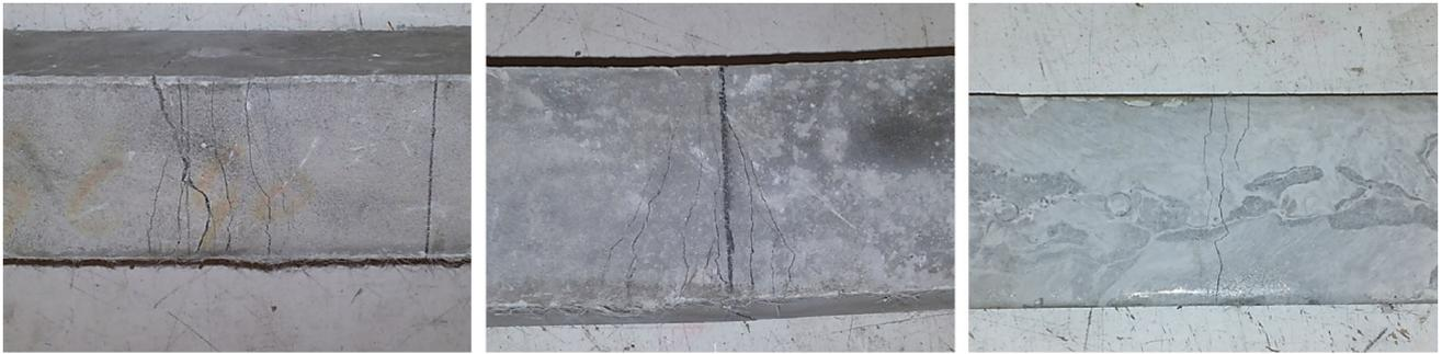
**Fig. 4** Multiple-cracking behavior as seen in the failed specimen.
