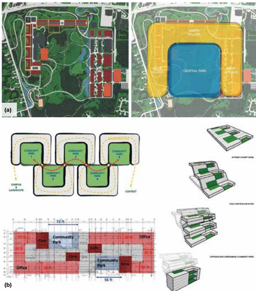
Fig. 3: Novartis facilities plans: (a) campus masterplan; and (b) Oncology Research Building stacking diagrams and floor plan
