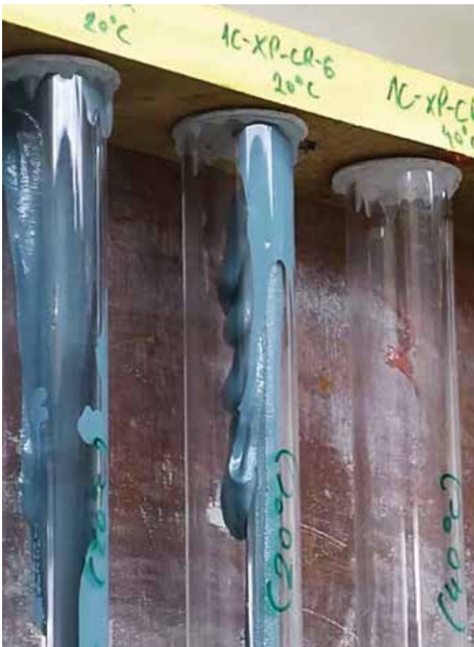
Fig. 5: Close-up of adhesive injection at the top of a large-diameter acrylic tube. The adhesive is not in contact with the full perimeter of the acrylic tube
