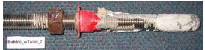
Fig. 2: End-cap installation with voids (Ocel et al. 7 )
