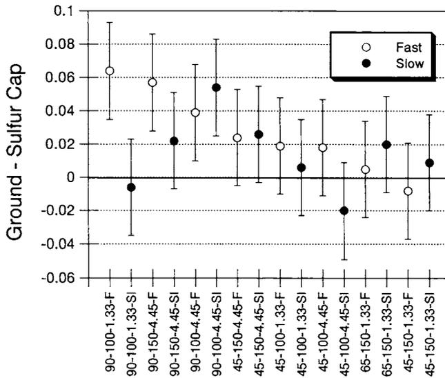
Fig. 8—Approximate 95 percent confidence intervals for effect of end condition (grinding-sulfur caps) for different strength, size, machine, speed combinations
