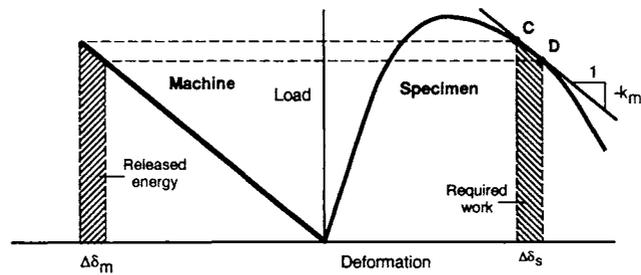
Fig. 4—Energy released by testing machine and work required to deform concrete specimen at different points along descending portion of load-deformation curve of specimen
