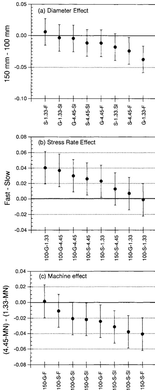
Fig. 9—Approximate 95 percent confidence intervals for effects of diameter, stress rate (speed), and machine for different settings of other factors
