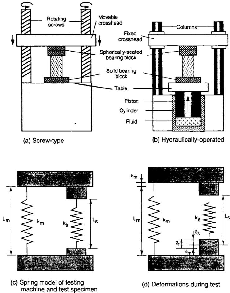
Fig. 3—(a) Schematic of screw-type testing machine; (b) schematic of hydraulically operated machine; (c) simplified spring model of specimen and testing machine; and (d) deformation of specimen and testing machine during testing
