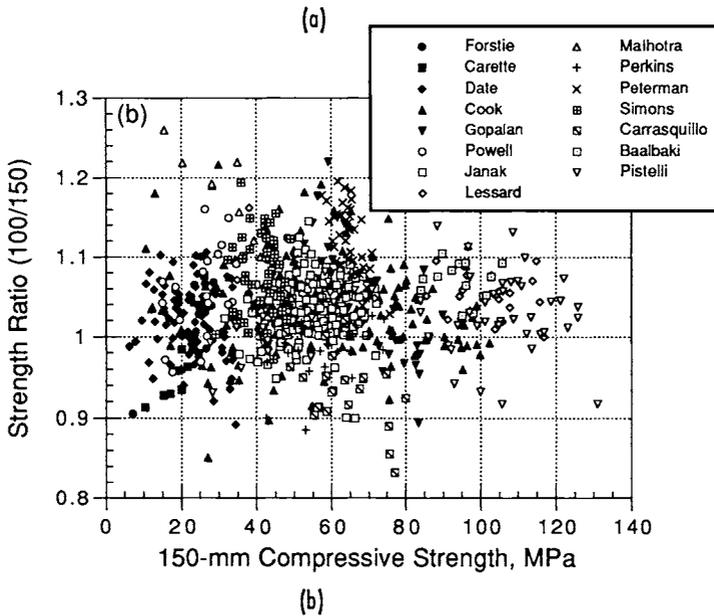
Fig. 1—(a) Comparison of compressive strength of 100- and 150-mm-diameter cylinders; (b) strength ratio as function of compressive strength of 150-mm cylinders
