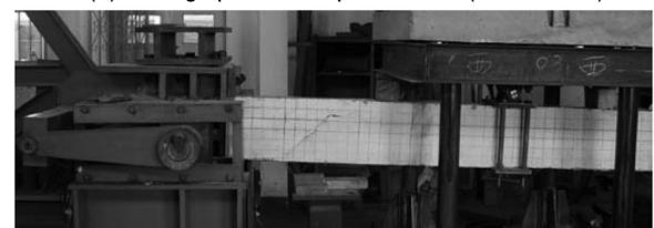
(b) Close-up of Specimen D3 at  $P = 54.6$  kN
