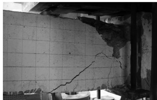
Fig. 7 Damage pattern of Specimen D4 at center column ( $P = 53.5$  kN).
