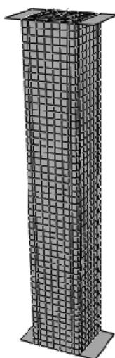
Fig. 3 Finite element model of FRP rebar reinforced concrete column.
