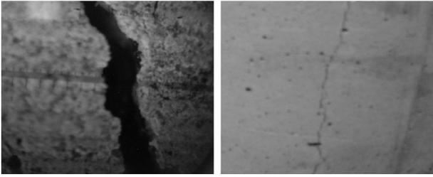
Fig. 7 Restrained shrinkage crack of RAPM 50% series.
