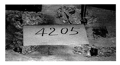
Figure 5.18 Typical Concrete Spalling after Reversed Loading
