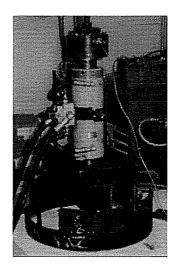
Figure 4.11 Test Setup for Single-Anchor Tension Tests
