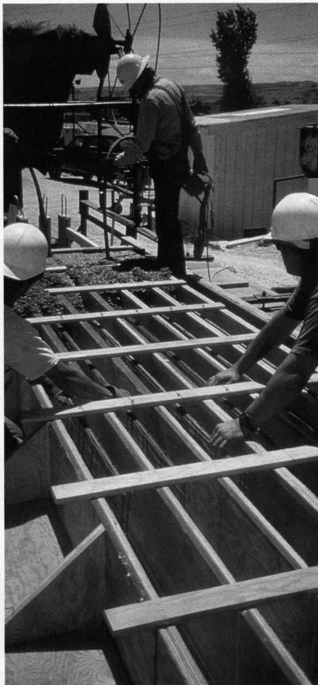
Fig. 12. Casting beam specimens (May 17, 1996).
