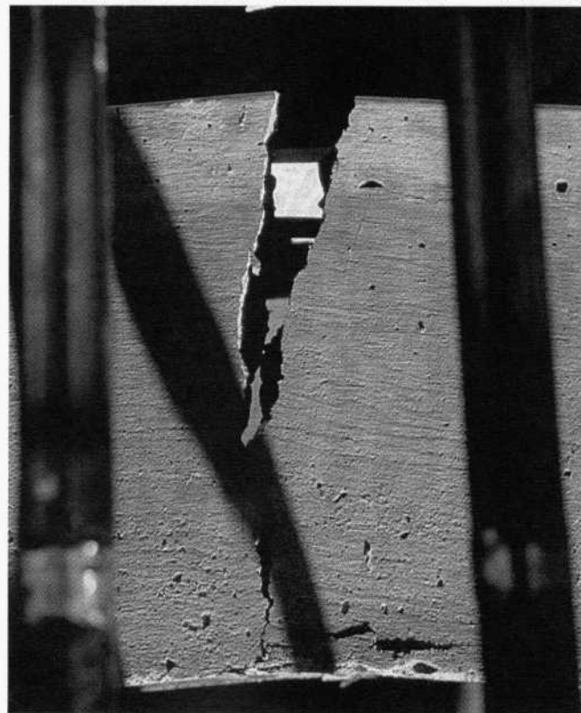
Fig. 28. Beam ER-2 (south) L = 4.58 ft (1.40 m). Bond failure occurred upon formation of first crack. Deflection = 0.1 in. (2.54 mm) prior to sudden failure. Strand slip at end = crack width (June 9, 1996).
