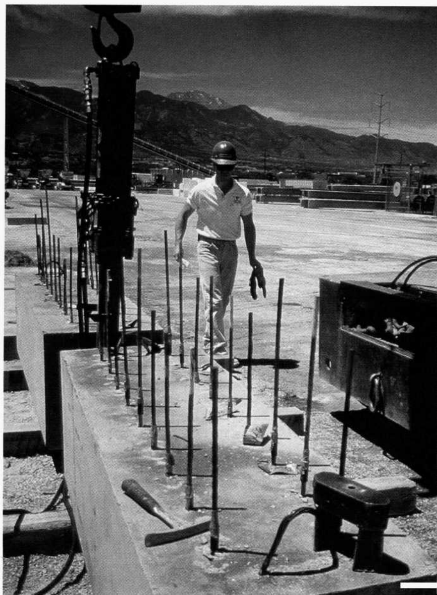
Fig. 17. Strand Groups D and ER pulled out 6 to 8 in. (152 to 203 mm) at 12 kips (53 kN) maximum load. Other groups exceeded 36 kips (160 kN) with less than 2 in. (51 mm) pull-out (May 18, 1996).
