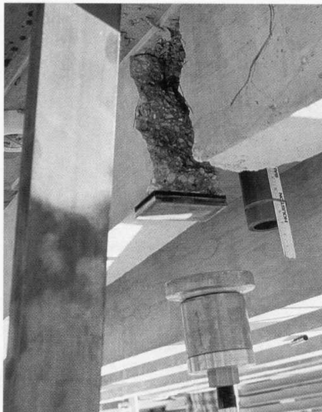
Fig. 27. Strand break, Beam TW-5 (north end). Energy release from 43 kip (191 kN) load in strand caused 6.08 ft (1.85 m) beam end to rebound 6 in. (152 mm) to north (June 8, 1996).
