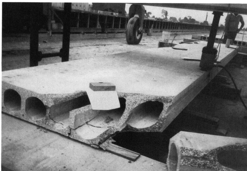
Fig. 14. Shear-torsion end failure for load at the quarter point (Test No. 14).
