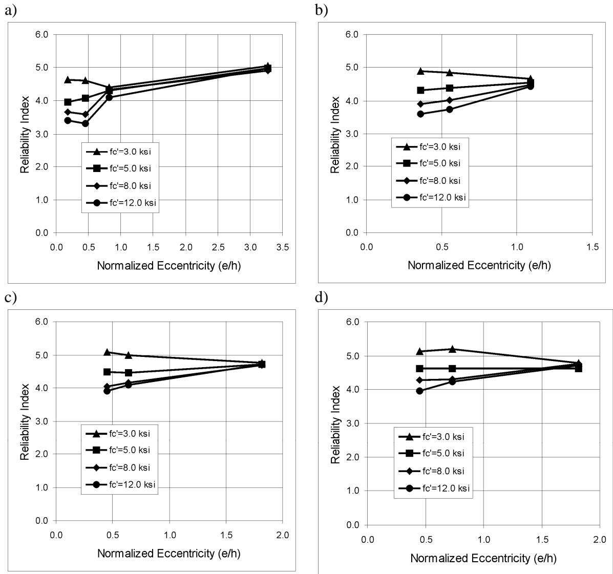
Figure 2-34. Reliability index versus load eccentricity; spiral columns, cast-in-place, resistance factor,  $\varphi = 0.70$ : a) reinforcement ratio,  $\rho = 1\%$ , b) reinforcement ratio,  $\rho = 2\%$ , c) reinforcement ratio,  $\rho = 3\%$ , d) reinforcement ratio,  $\rho = 4\%$ ,
