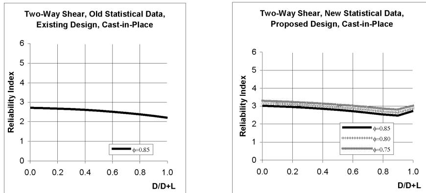
Fig. 3-2. Reliability Indices for R/C Slab Made of Ordinary Concrete for D+L Load Combination (for slab thickness equal to 6 in and without shear reinforcement).
