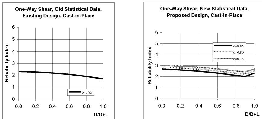
Fig. 3-5. Reliability Indices for R/C Foundation Beam Made of Ordinary Concrete for D+L Load Combination (for foundation depth equal to 36 in and without shear reinforcement).
