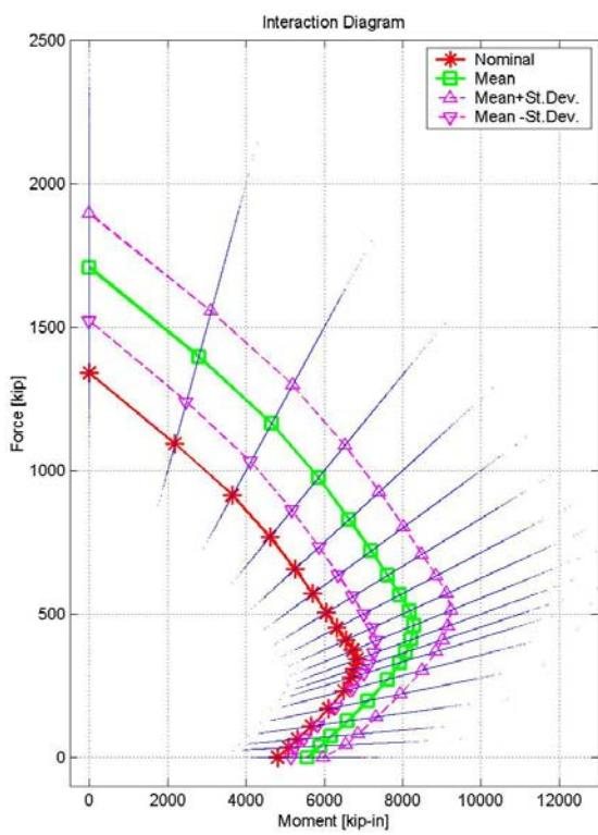
Figure 2-7. Mean and Nominal Interaction Diagrams (for concrete strength of 3 ksi, tied columns, cast-in-place).
