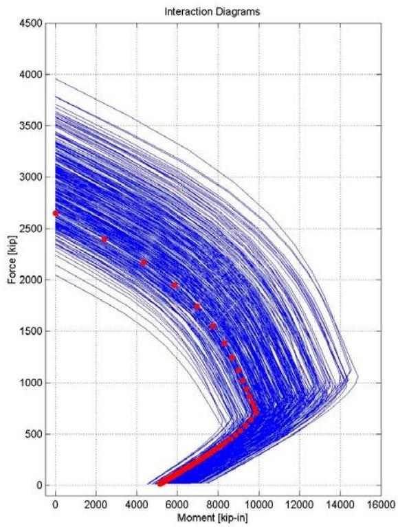
Figure 2-6. Simulated Interaction Diagrams (for concrete strength of 8 ksi, tied columns, cast-in-place), Red Dots are Nominal Values.
