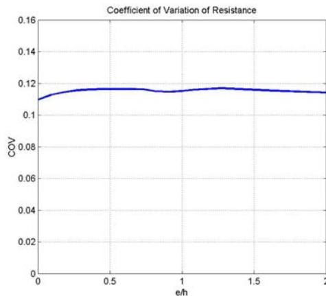
Figure 2-15. Coefficient of Variation of Resistance (calculated for tied columns cast-in-place made of concrete with strength of 3 ksi ).
