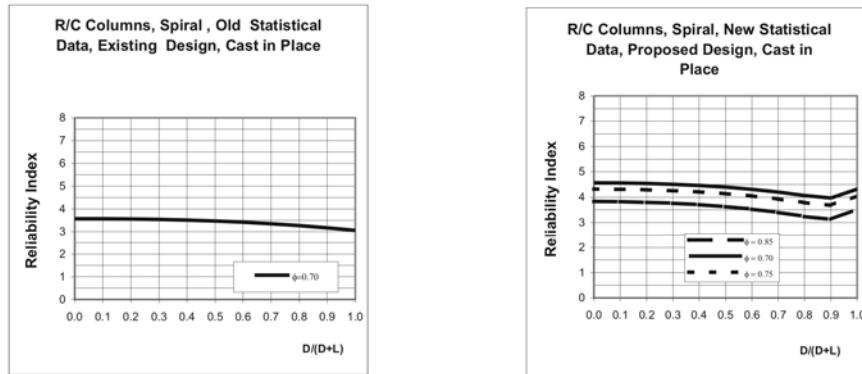
Reliability Indices Calculated for R/C Column Made of Ordinary Concrete for D+L Load Combination
