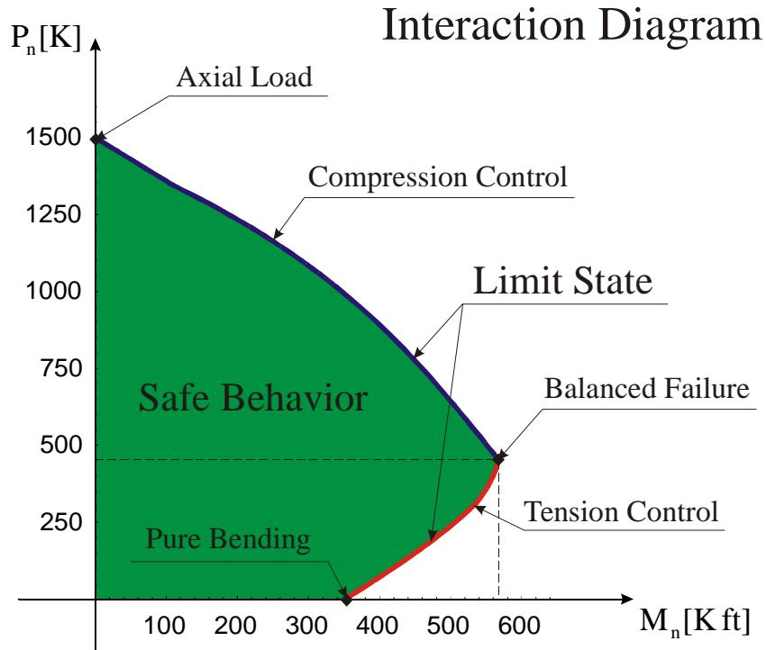
Figure 2-1. Interaction diagram for eccentrically loaded columns.
