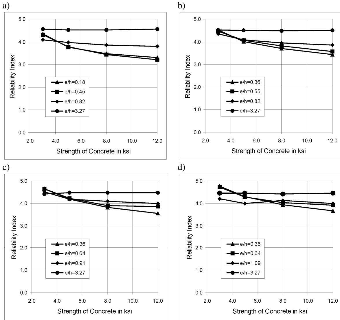
Figure 2-29. Reliability index versus strength of concrete; tied columns, cast-in-place, for  $h/b = 1.57$  and resistance factor,  $\varphi = 0.70$ : a) reinforcement ratio,  $\rho = 1\%$ , b) reinforcement ratio,  $\rho = 2\%$ , c) reinforcement ratio,  $\rho = 3\%$ , d) reinforcement ratio,  $\rho = 4\%$ ,
