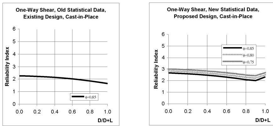
Fig. 3-4. Reliability Indices for R/C Foundation Beam Made of Ordinary Concrete for D+L Load Combination (for foundation depth equal to 12 in and without shear reinforcement).
