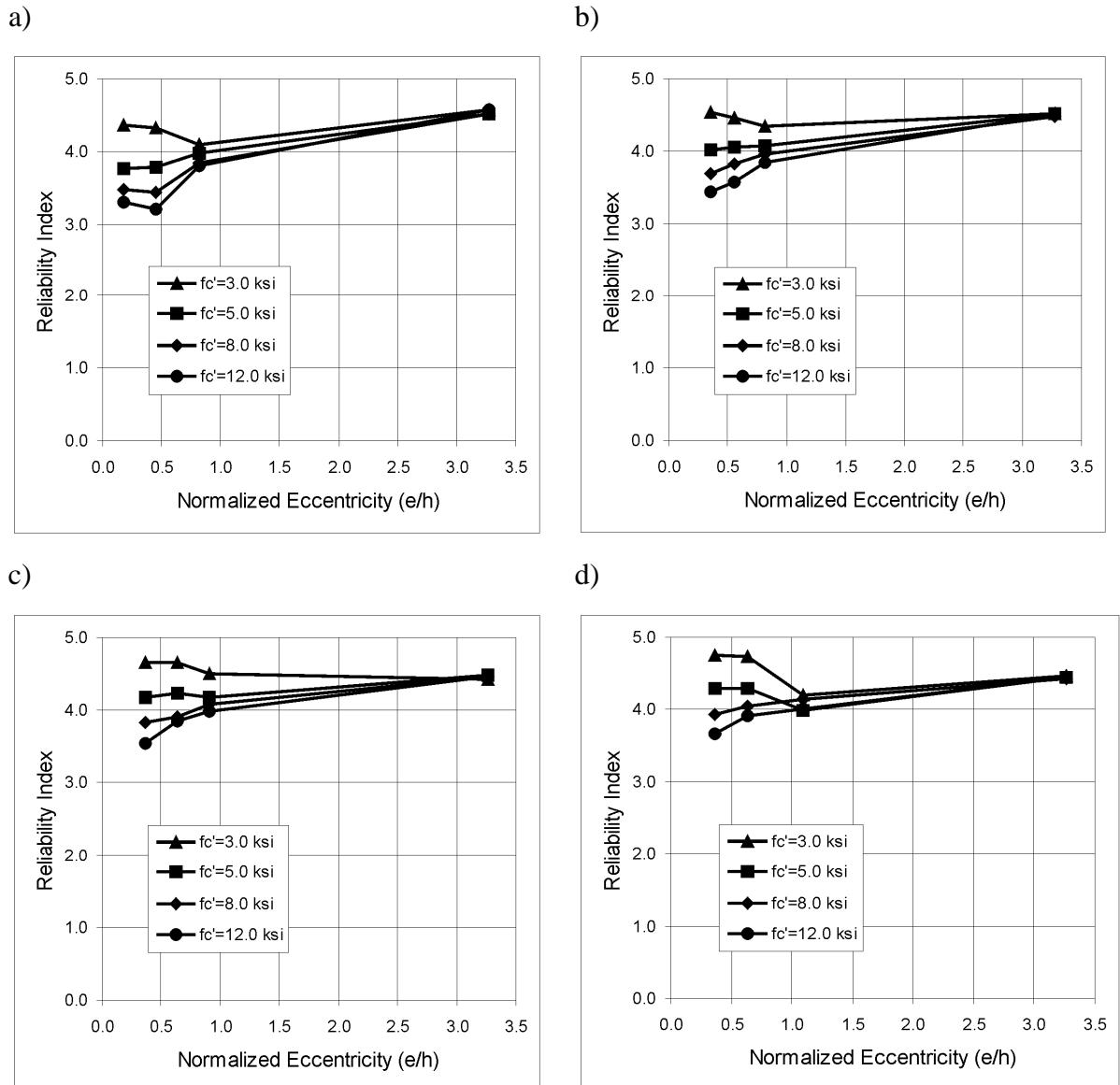
Figure 2-30. Reliability index versus load eccentricity; tied columns, cast-in-place, for  $h/b = 1.57$  and resistance factor,  $\varphi = 0.70$ : a) reinforcement ratio,  $\rho = 1\%$ , b) reinforcement ratio,  $\rho = 2\%$ , c) reinforcement ratio,  $\rho = 3\%$ , d) reinforcement ratio,  $\rho = 4\%$ ,
