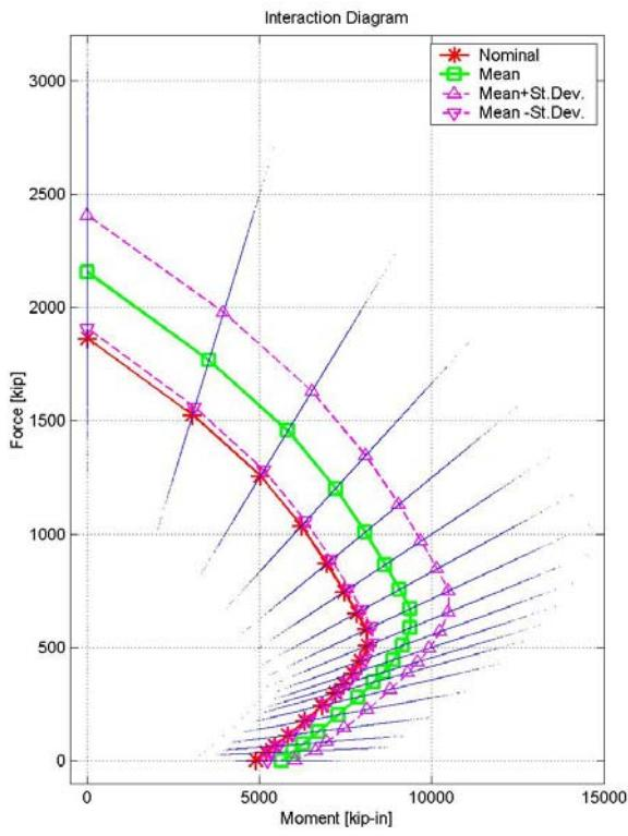
Figure 2-8. Mean and Nominal Interaction Diagrams (for concrete strength of 5 ksi, tied columns, cast-in-place).
