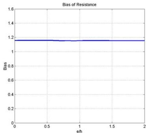
Figure 2-12. Bias Factor of Resistance (calculated for tied columns cast-in-place made of concrete with strength of 5 ksi).
