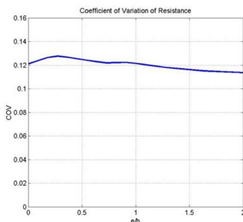
Figure 2-17. Coefficient of Variation of Resistance (calculated for tied columns cast-in-place made of concrete with strength of 8 ksi ).
