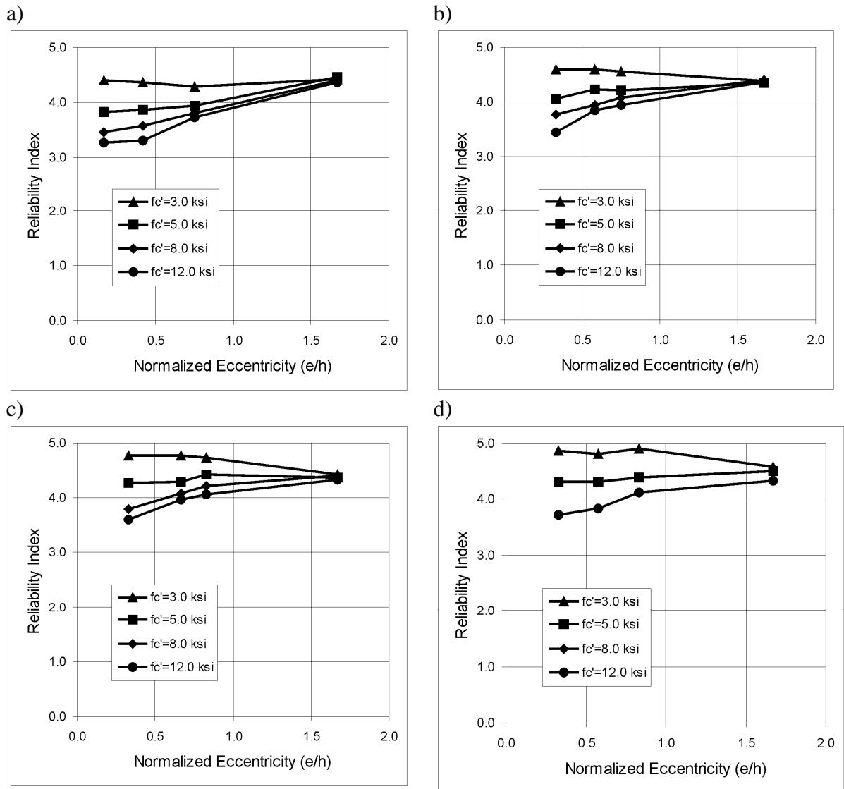
Figure 2-32. Reliability index versus load eccentricity; tied columns, cast-in-place, for  $h/b = 2.0$  and resistance factor,  $\varphi = 0.70$ : a) reinforcement ratio,  $\rho = 1\%$ , b) reinforcement ratio,  $\rho = 2\%$ , c) reinforcement ratio,  $\rho = 3\%$ , d) reinforcement ratio,  $\rho = 4\%$ ,
