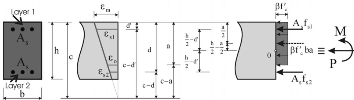
Figure 2-2. Strain and Stress Distribution in Cross Section of an Eccentrically Loaded Column.
