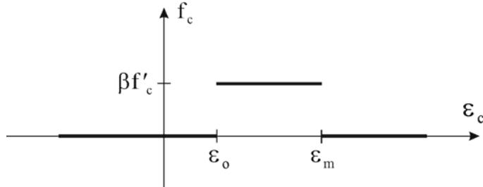
Figure 2-4. Stress vs. Strain Relationship for Concrete.
