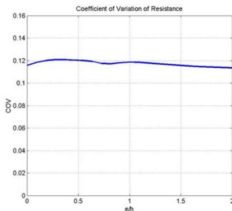
Figure 2-16. Coefficient of Variation of Resistance (calculated for tied columns cast-in-place made of concrete with strength of 5 ksi ).
