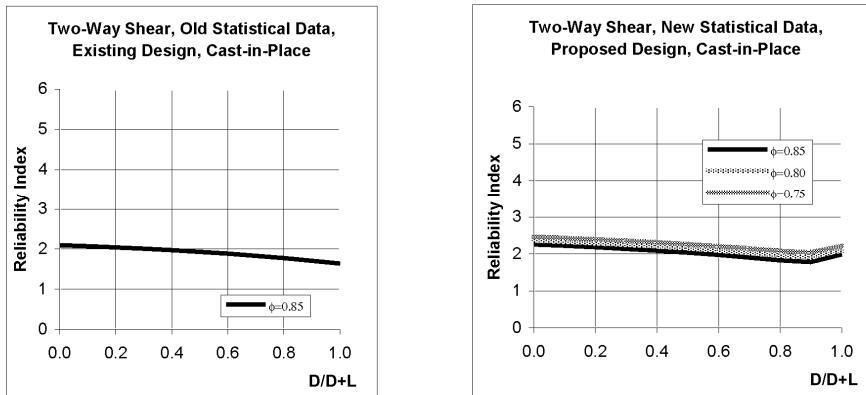
Fig.3-1. Reliability Indices Calculated for R/C Slab Made of Ordinary Concrete for D+L Load Combination (for slab thickness equal to 4 in and without shear reinforcement).
