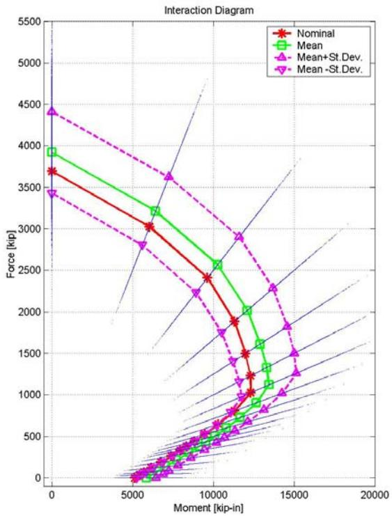
Figure 2-10. Mean and Nominal Interaction Diagrams (for concrete strength of 12 ksi, tied columns, cast-in-place).
