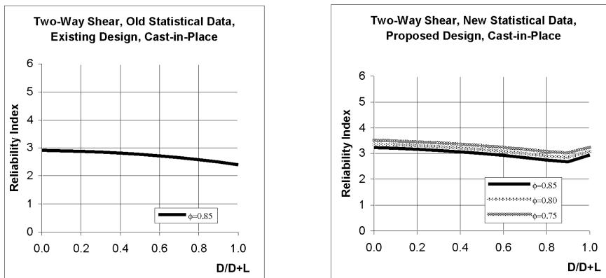
Fig. 3-3. Reliability Indices for R/C Slab Made of Ordinary Concrete for D+L Load Combination (for slab thickness equal to 8 in and without shear reinforcement).
