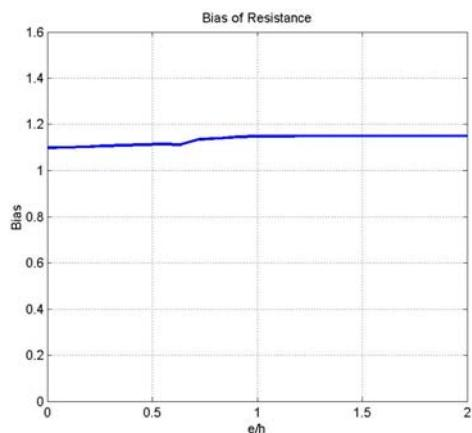
Figure 2-13. Bias Factor of Resistance (calculated for tied columns cast-in-place made of concrete with strength of 8 ksi).
