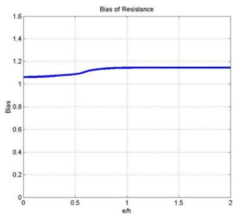
Figure 2-14. Bias Factor of Resistance (calculated for tied columns cast-in-place made of concrete with strength of 12 ksi).
