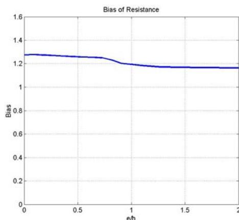
Figure 2-11. Bias Factor of Resistance (calculated for tied columns cast-in-place made of concrete with strength of 3 ksi).
