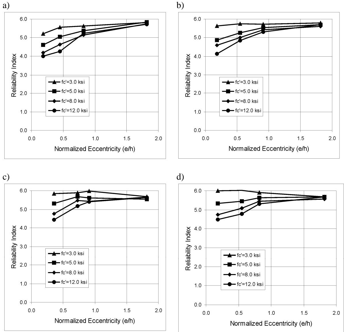
Figure 2-36. Reliability index versus load eccentricity; tied columns, plant cast, for  $h/b = 1.57$  and resistance factor,  $\varphi = 0.70$ : a) reinforcement ratio,  $\rho = 1\%$ , b) reinforcement ratio,  $\rho = 2\%$ , c) reinforcement ratio,  $\rho = 3\%$ , d) reinforcement ratio,  $\rho = 4\%$ ,
