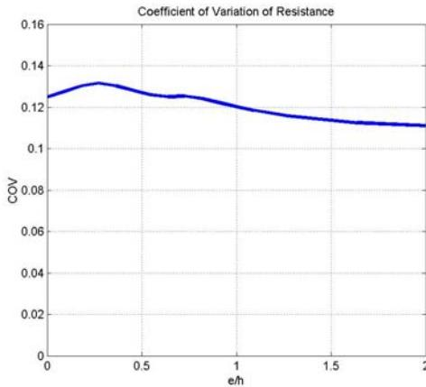
Figure 2-18. Coefficient of Variation of Resistance (calculated for tied columns cast-in-place made of concrete with strength of 12 ksi ).
