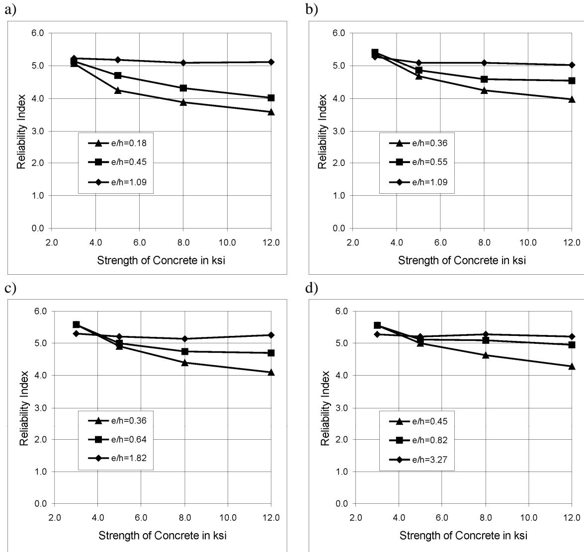
Figure 2-39. Reliability index versus strength of concrete; spiral columns, plant cast, for resistance factor,  $\varphi = 0.70$ : a) reinforcement ratio,  $\rho = 1\%$ , b) reinforcement ratio,  $\rho = 2\%$ , c) reinforcement ratio,  $\rho = 3\%$ , d) reinforcement ratio,  $\rho = 4\%$ ,
