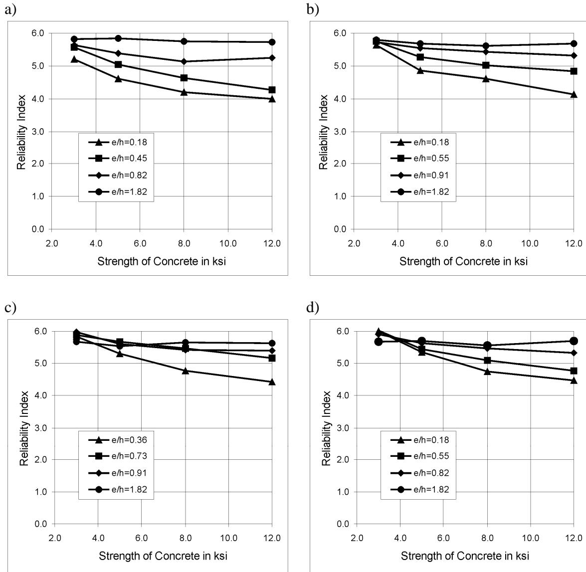
Figure 2-35. Reliability index versus strength of concrete; tied columns, plant cast, for  $h/b = 1.57$  and resistance factor,  $\varphi = 0.70$ : a) reinforcement ratio,  $\rho = 1\%$ , b) reinforcement ratio,  $\rho = 2\%$ , c) reinforcement ratio,  $\rho = 3\%$ , d) reinforcement ratio,  $\rho = 4\%$ ,
