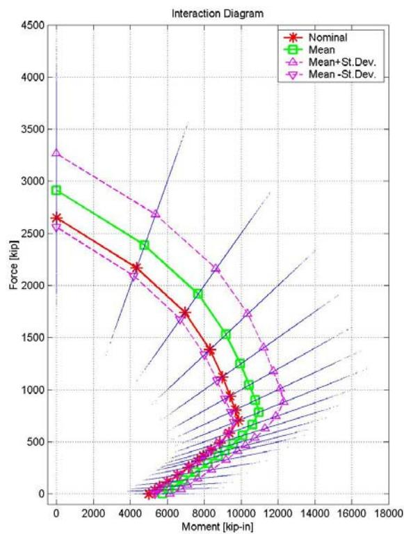
Figure 2-9. Mean and Nominal Interaction Diagrams (for concrete Strength of 8 ksi, tied columns, cast-in-place).
