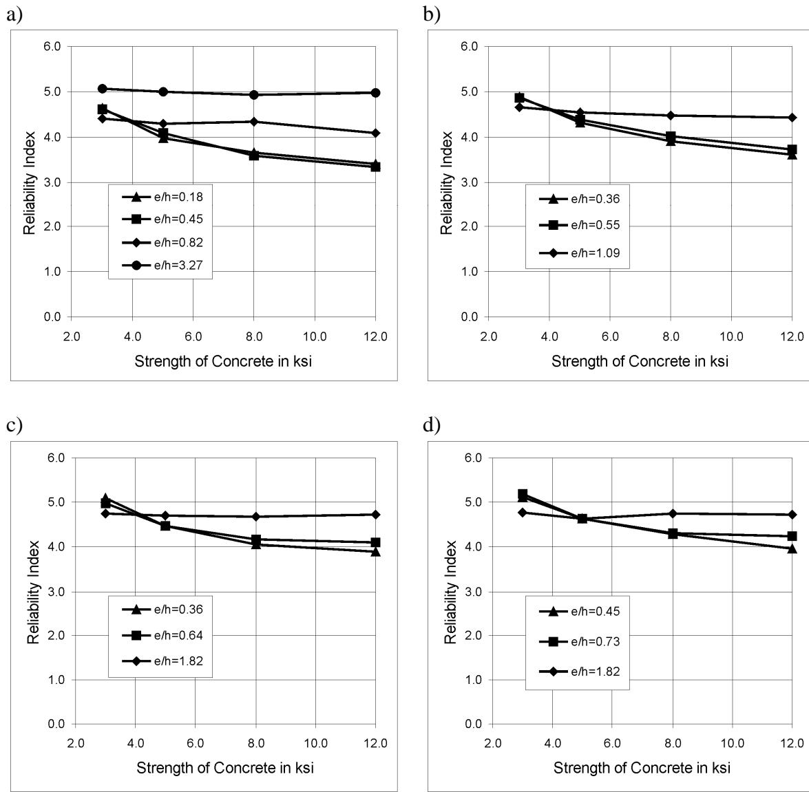
Figure 2-33. Reliability index versus strength of concrete; spiral columns, cast-in-place, for resistance factor,  $\varphi = 0.70$ : a) reinforcement ratio,  $\rho = 1\%$ , b) reinforcement ratio,  $\rho = 2\%$ , c) reinforcement ratio,  $\rho = 3\%$ , d) reinforcement ratio,  $\rho = 4\%$ ,
