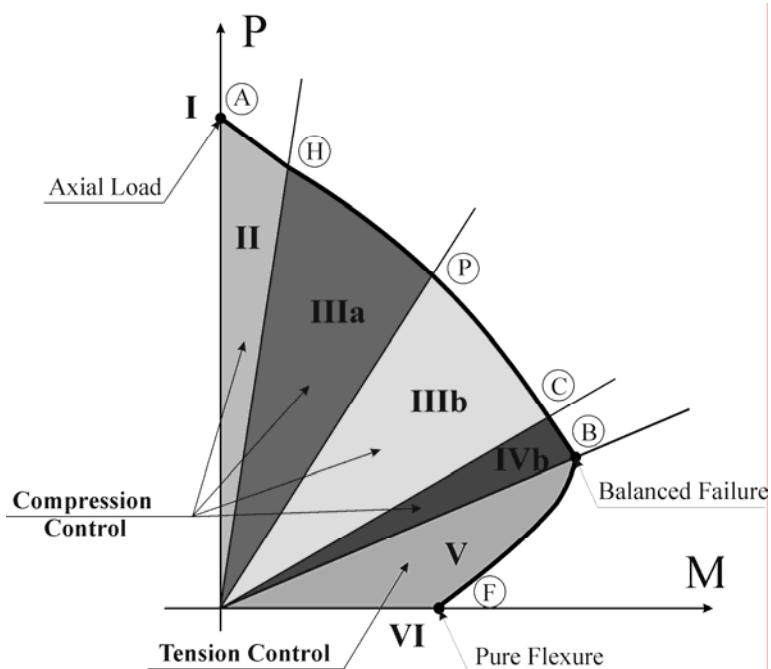
Figure 2-5. Interaction Diagram for Eccentrically Compressed Columns;
