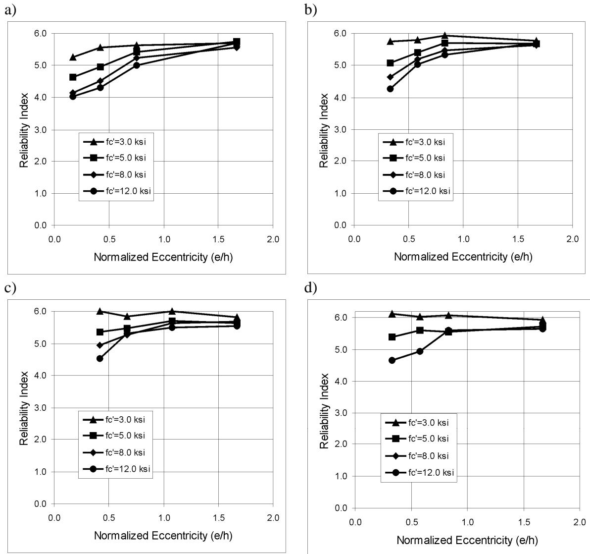
Figure 2-38. Reliability index versus load eccentricity; tied columns, plant cast, for  $h/b = 2.0$  and resistance factor,  $\varphi = 0.70$ : a) reinforcement ratio,  $\rho = 1\%$ , b) reinforcement ratio,  $\rho = 2\%$ , c) reinforcement ratio,  $\rho = 3\%$ , d) reinforcement ratio,  $\rho = 4\%$ ,
