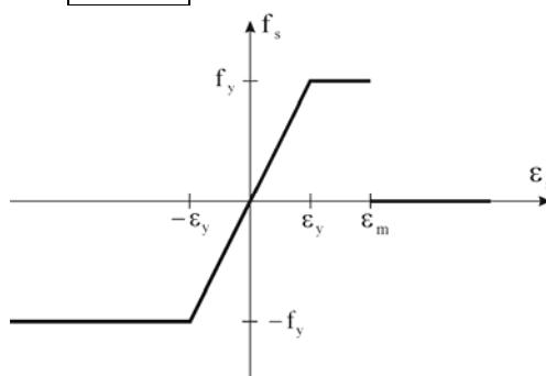
Figure 2-3. Stress vs. Strain Relationship for Reinforcing Steel.
