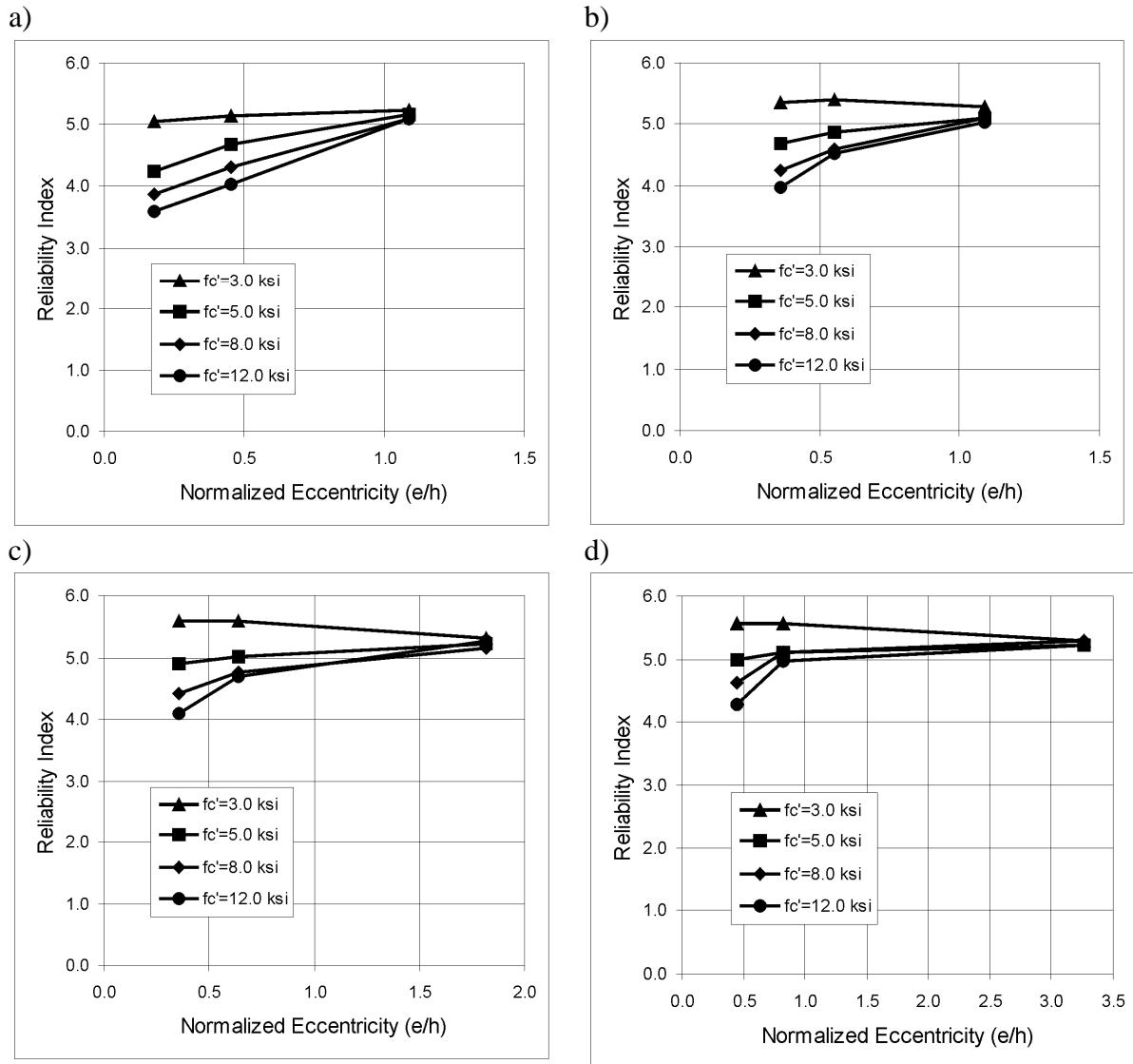
Figure 2-40. Reliability index versus load eccentricity; spiral columns, plant cast, for resistance factor,  $\varphi = 0.70$ : a) reinforcement ratio,  $\rho = 1\%$ , b) reinforcement ratio,  $\rho = 2\%$ , c) reinforcement ratio,  $\rho = 3\%$ , d) reinforcement ratio,  $\rho = 4\%$ ,
