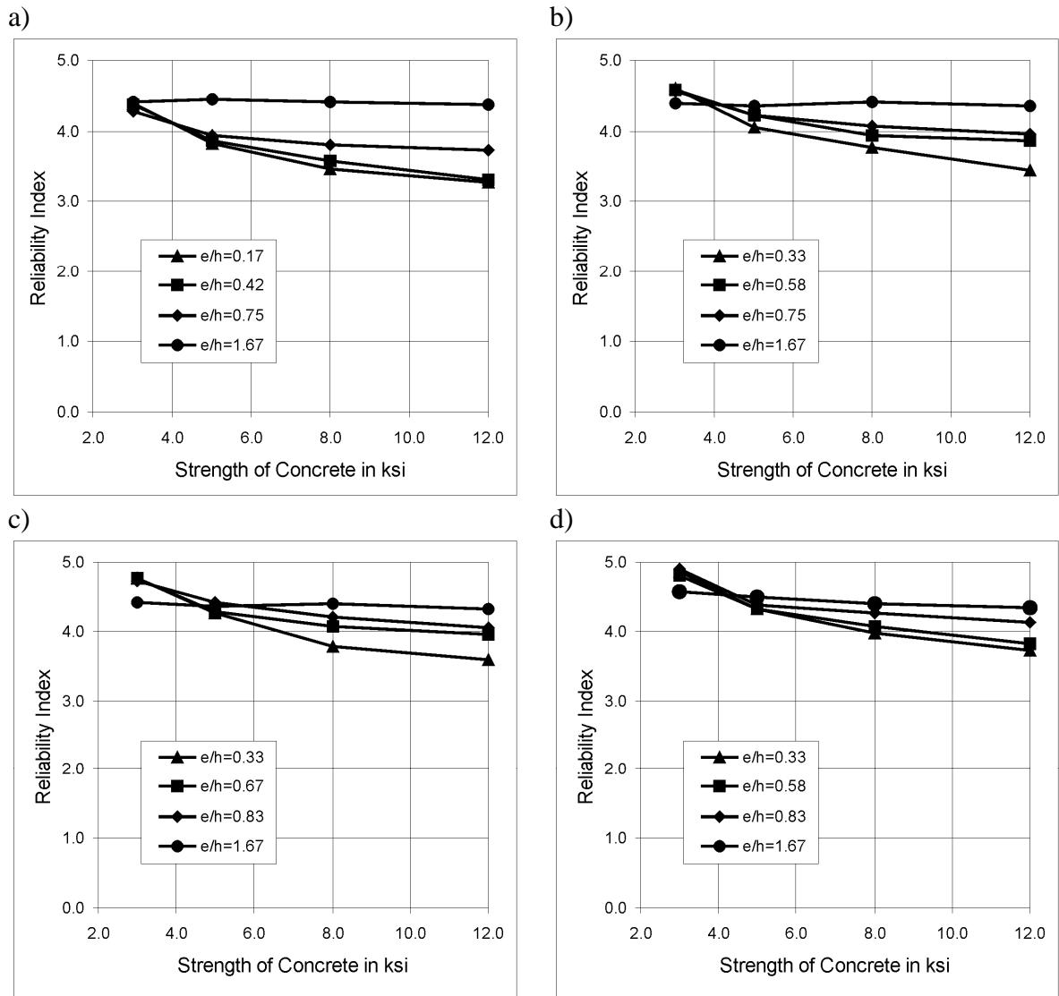
Figure 2-31. Reliability index versus strength of concrete; tied columns, cast-in-place, for  $h/b = 2.0$  and resistance factor,  $\varphi = 0.70$ : a) reinforcement ratio,  $\rho = 1\%$ , b) reinforcement ratio,  $\rho = 2\%$ , c) reinforcement ratio,  $\rho = 3\%$ , d) reinforcement ratio,  $\rho = 4\%$ ,
