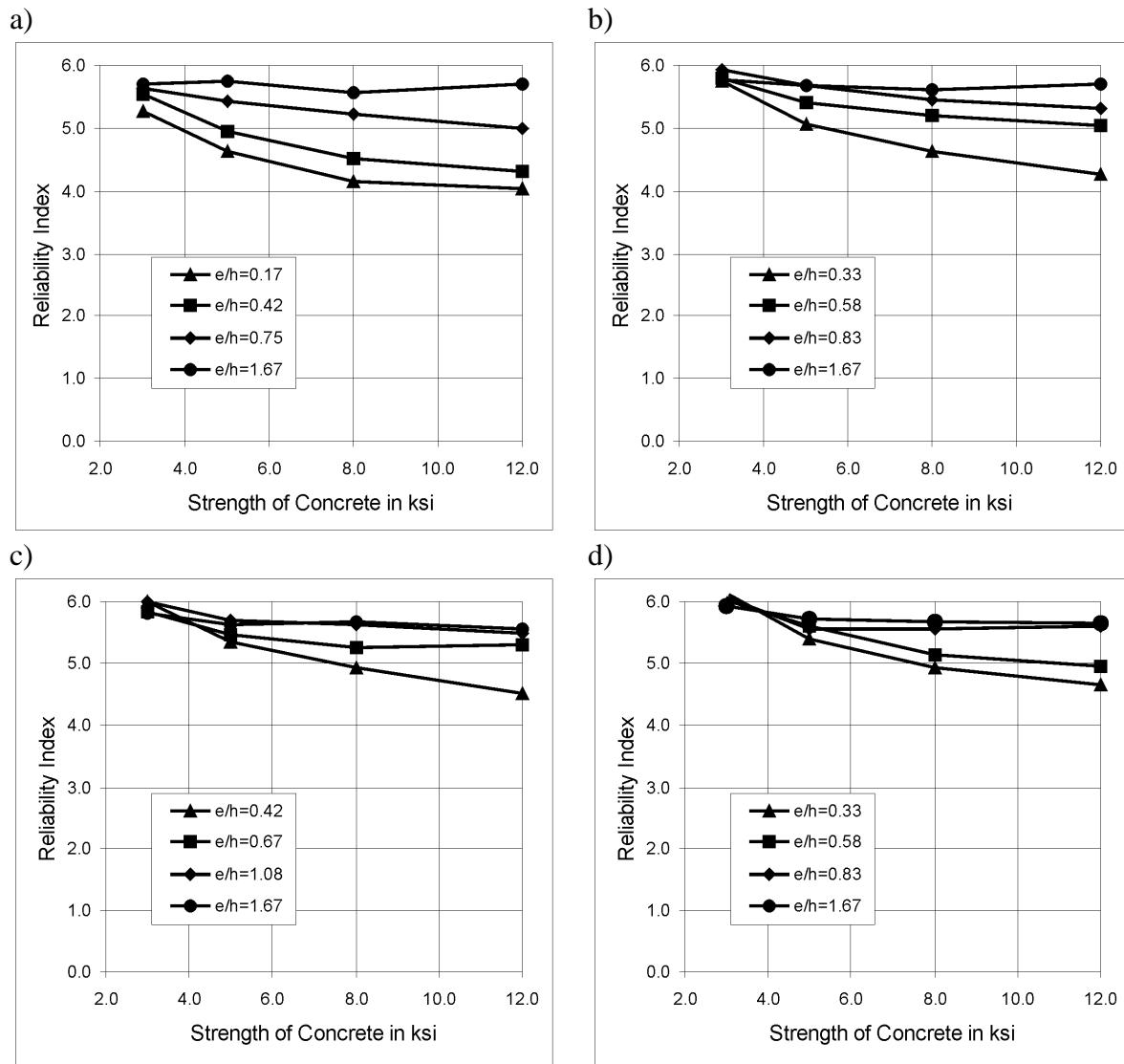
Figure 2-37. Reliability index versus strength of concrete; tied columns, plant cast, for  $h/b = 2.0$  and resistance factor,  $\varphi = 0.70$ : a) reinforcement ratio,  $\rho = 1\%$ , b) reinforcement ratio,  $\rho = 2\%$ , c) reinforcement ratio,  $\rho = 3\%$ , d) reinforcement ratio,  $\rho = 4\%$ ,
