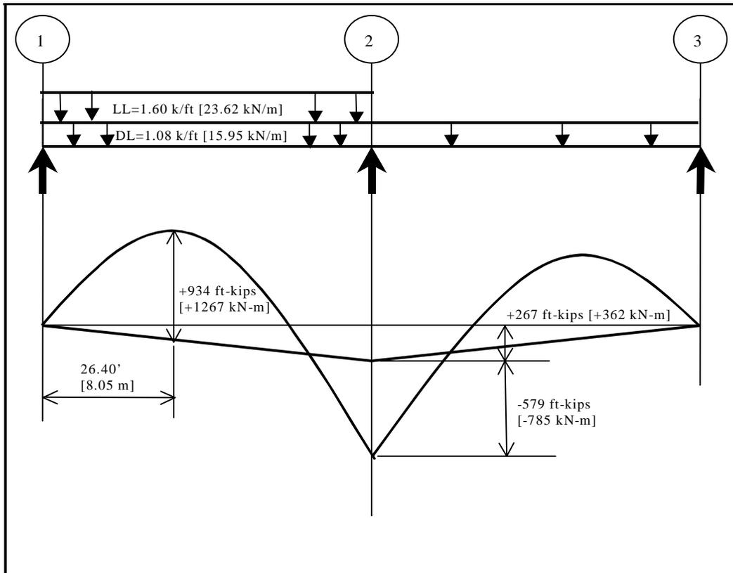
Fig. 15 - Maximum elastic positive moment in span 1-2
