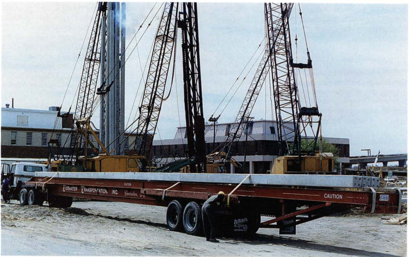
Fig. 4.1. Expandable trailer for transporting piles up to 110 ft (33.5 m) long.
