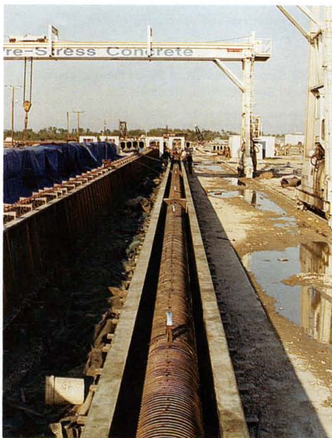
Fig. 2.12. Congestion with heavy spiral reinforcement.
