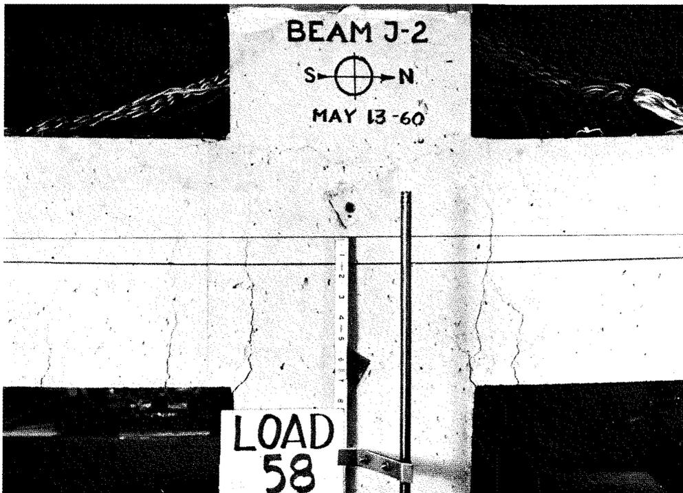
**Fig. 5-26. Beam-column connection at first visible crushing.**
