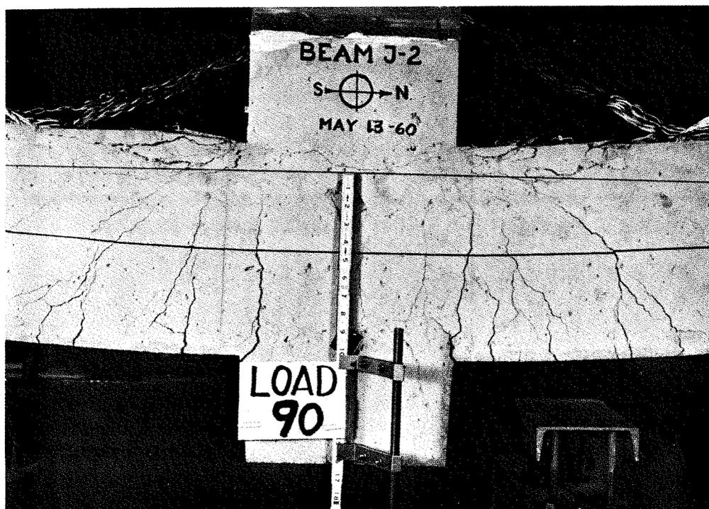
**Fig. 5-28. Beam-column connection at about eight times the yield deflection.**
