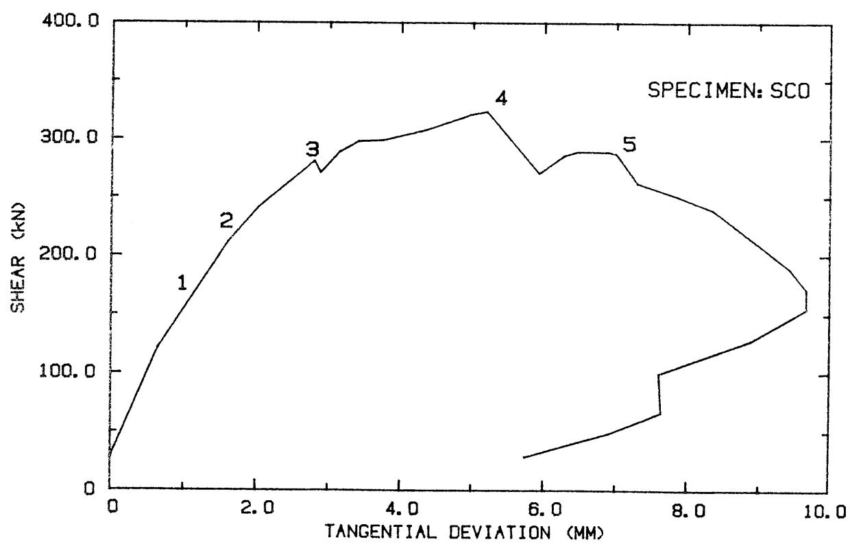
Fig. 3.1: Load-displacement curves for specimen SCO.
