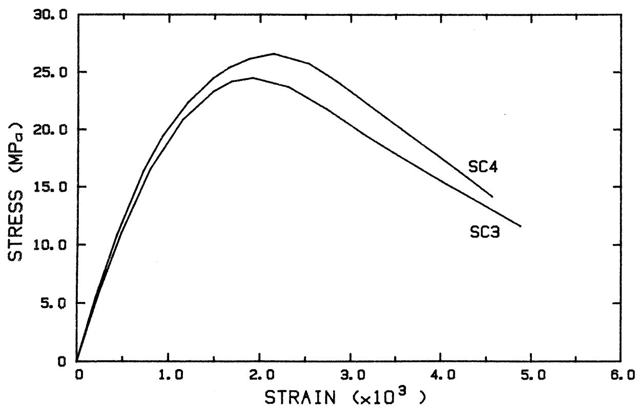
Fig. 2.10: Stress-strain characteristics of concrete.
