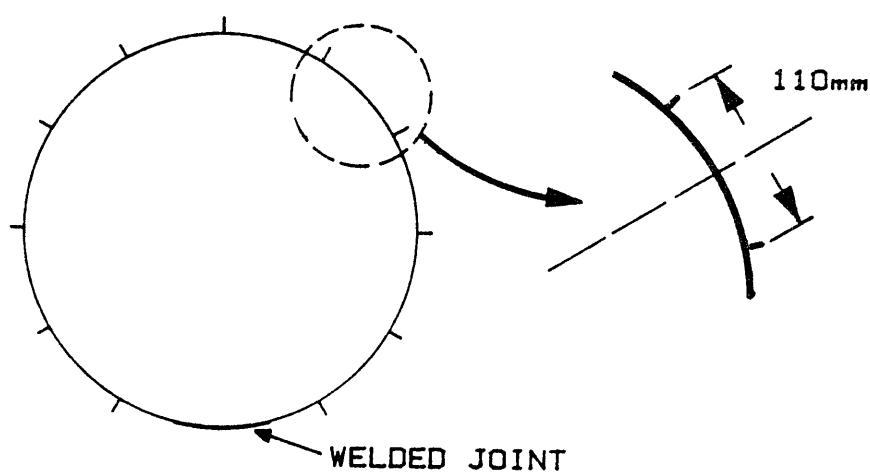
Fig. 2.13: Typical instrumented hoop.
