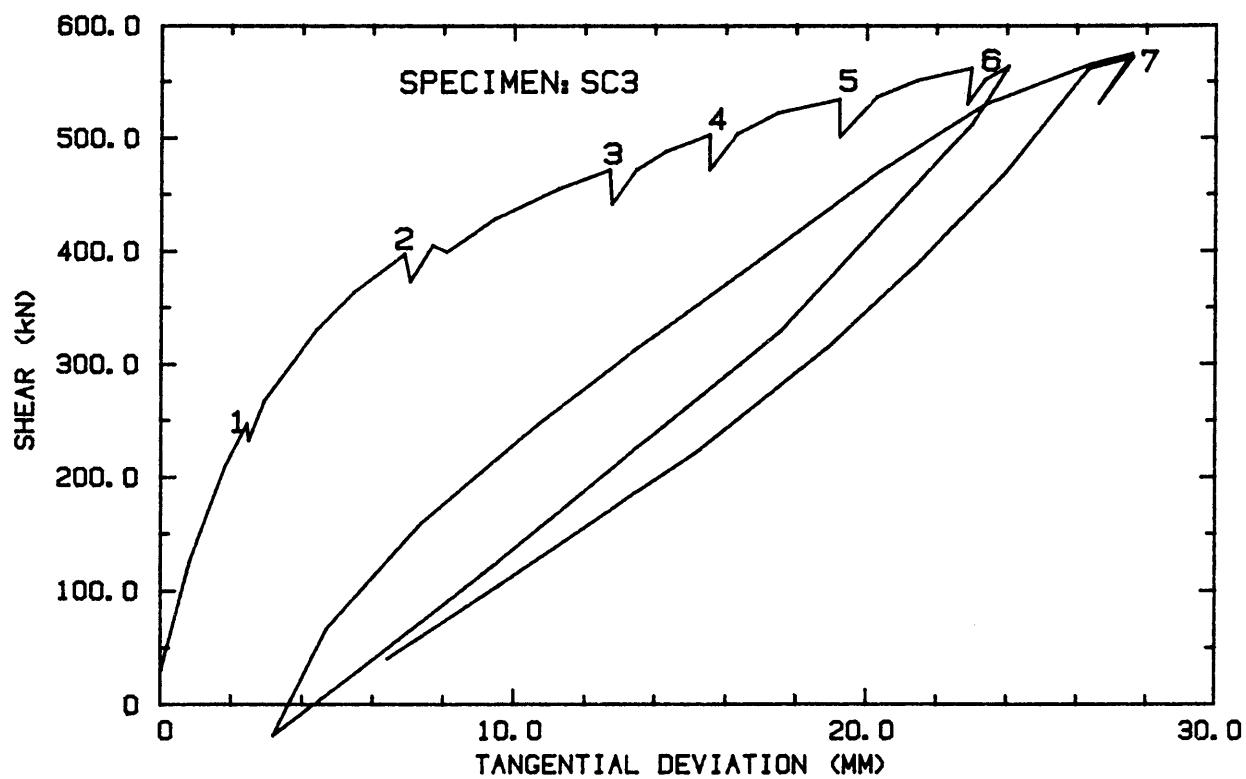
Fig. 3.7: Load-displacement curves for specimen SC3.
