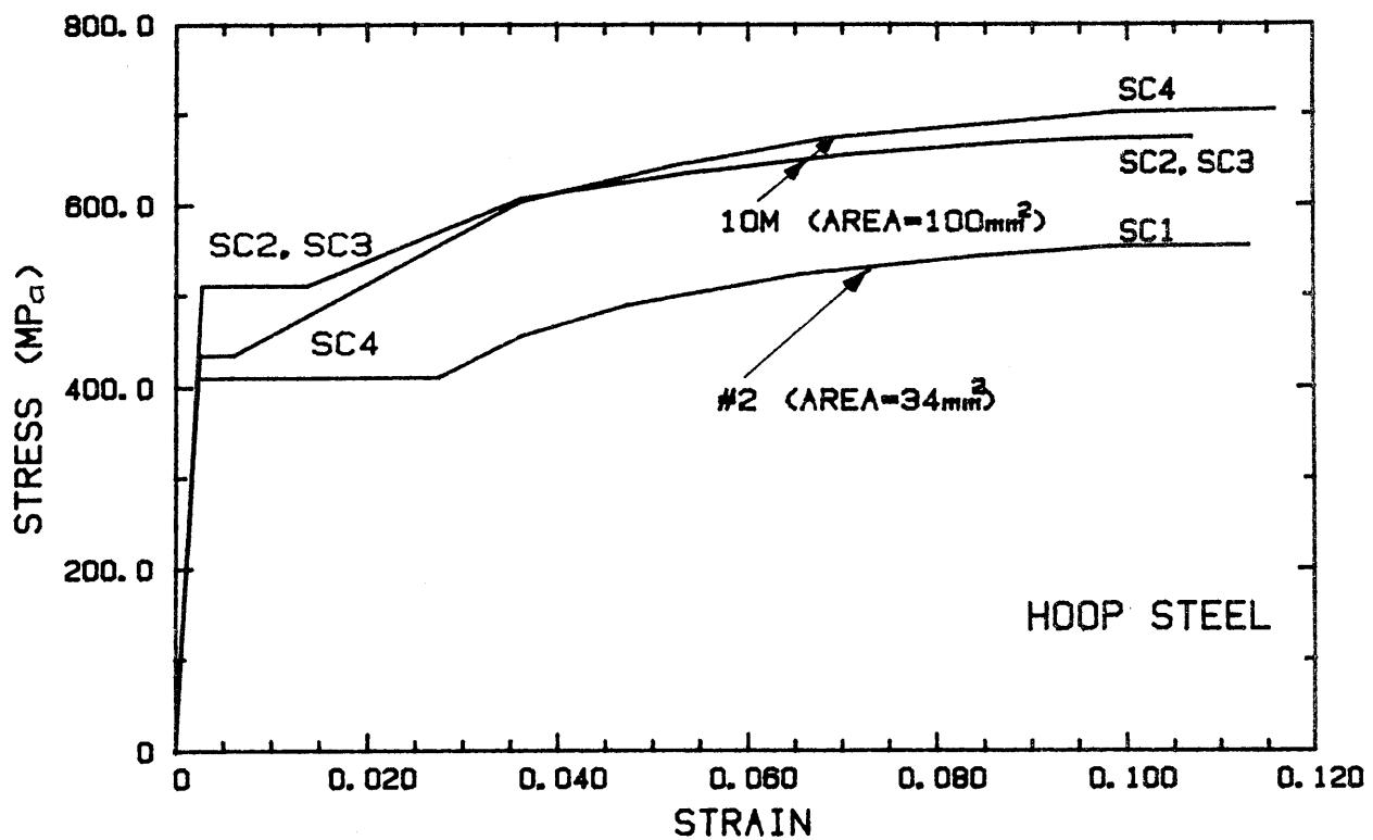
Fig. 2.8: Typical stress-strain curves for hoop steel.
