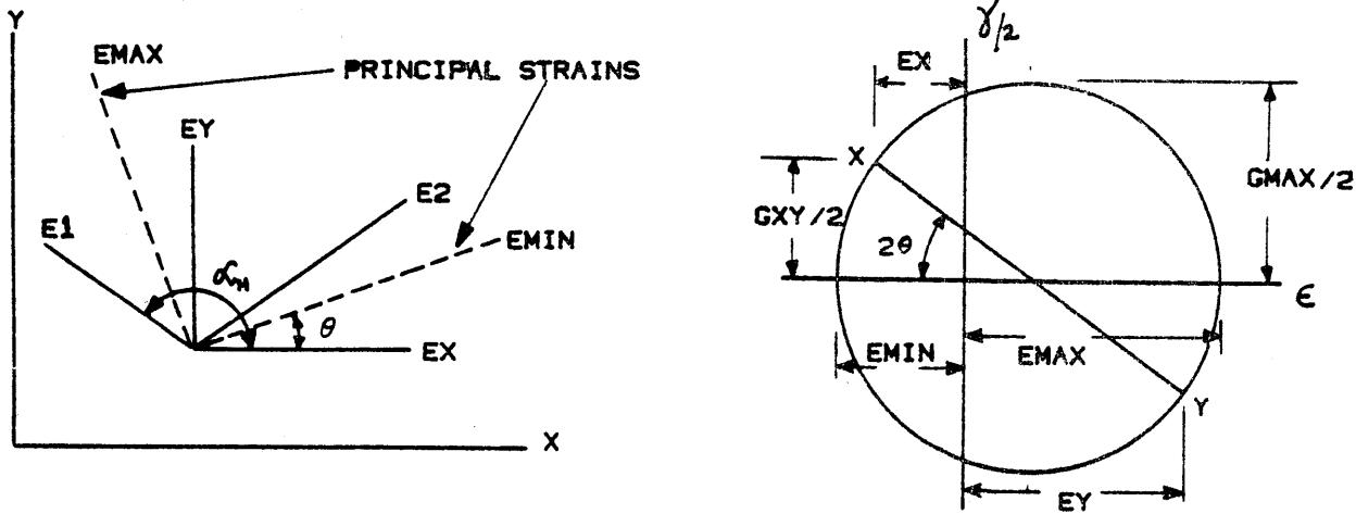
Fig. B.1: Strains in a typical grid
