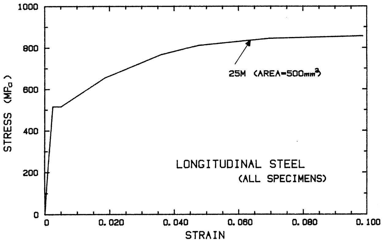
Fig. 2.9: Typical stress-strain curve for longitudinal steel.
