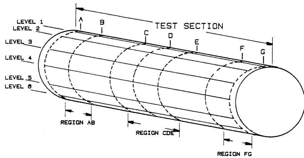
Fig. 2.14: Position of instrumented hoops in the specimen.
