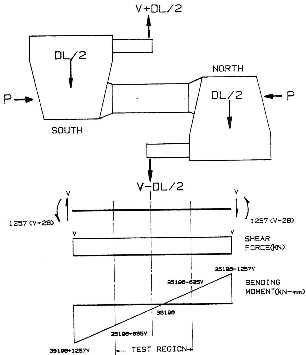
Fig. 2.4: Assumed moment and shear diagrams for test region.
