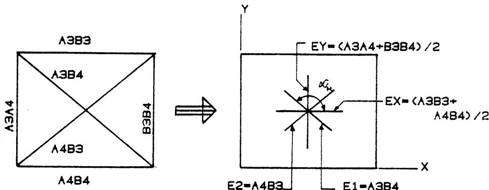
Fig. 4.3(b): Strains measured in a typical grid element.
