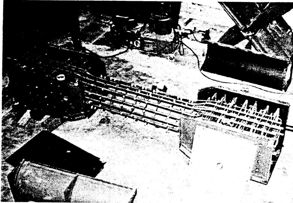
Fig. 2.7: Typical reinforcing cage for the test specimens.
