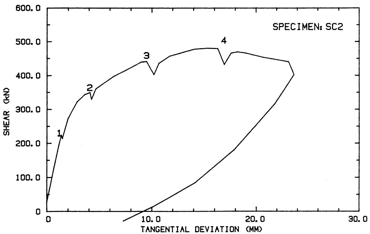
Fig. 3.5: Load-displacement curves for specimen SC2.
