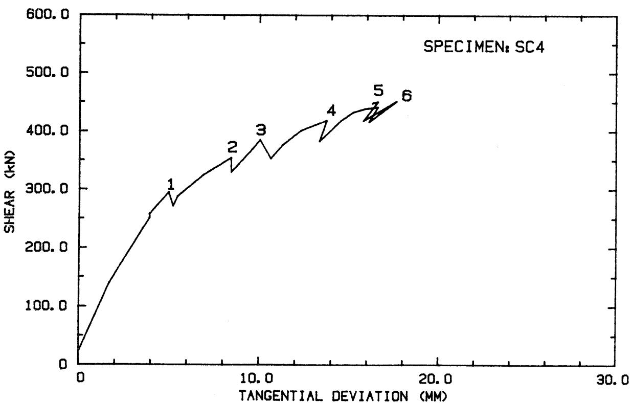
Fig. 3.9: Load-displacement curves for specimen SC4.
