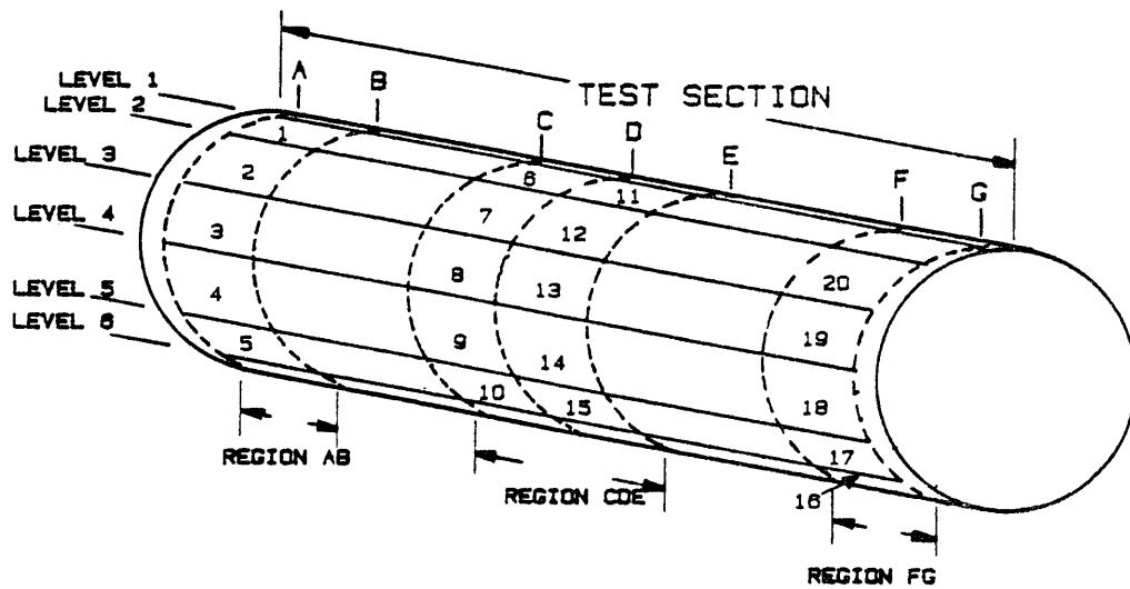
Fig. 4.3(a): Grid elements on which readings were taken.
