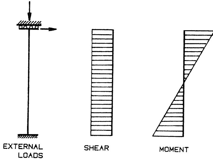
Fig. 2.1: Loading simulated during test.
