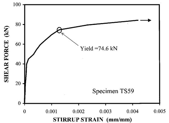
Fig. 4—Load-stirrup strain curve for TS59.
