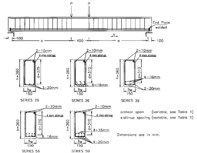
Fig. 2—Dimensions and reinforcements of test specimens.
