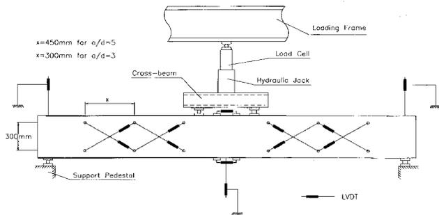
Fig. 3—Test setup and instrumentation (external).
