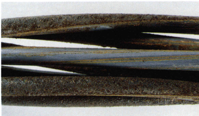
Photo 8. Strand surface before cleaning.
