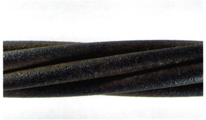
Photo 7A. Strand surface after cleaning.
