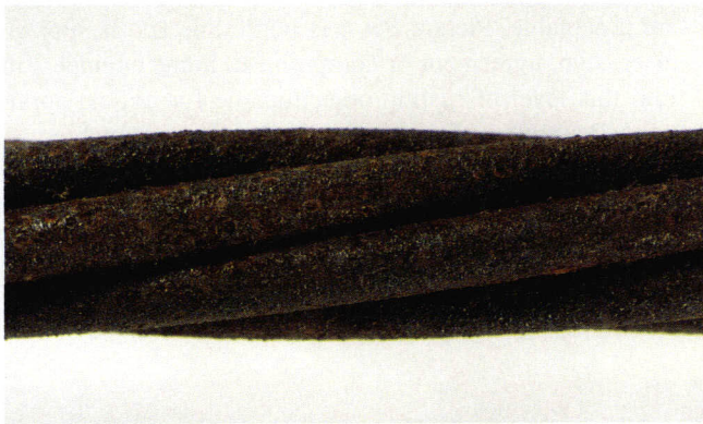
Photo 7. Strand surface before cleaning.
