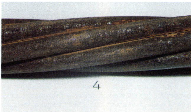
Photo 4. Strand surface before cleaning.
