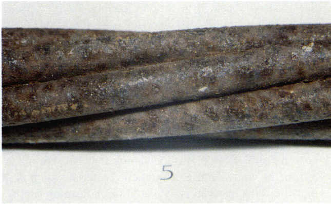
Photo 5. Strand surface before cleaning.
