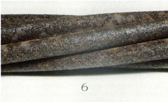
Photo 6. Strand surface before cleaning.
