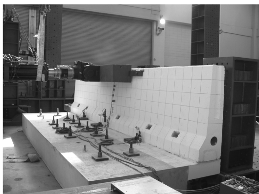
Fig. 5 Static test of concrete barrier.
