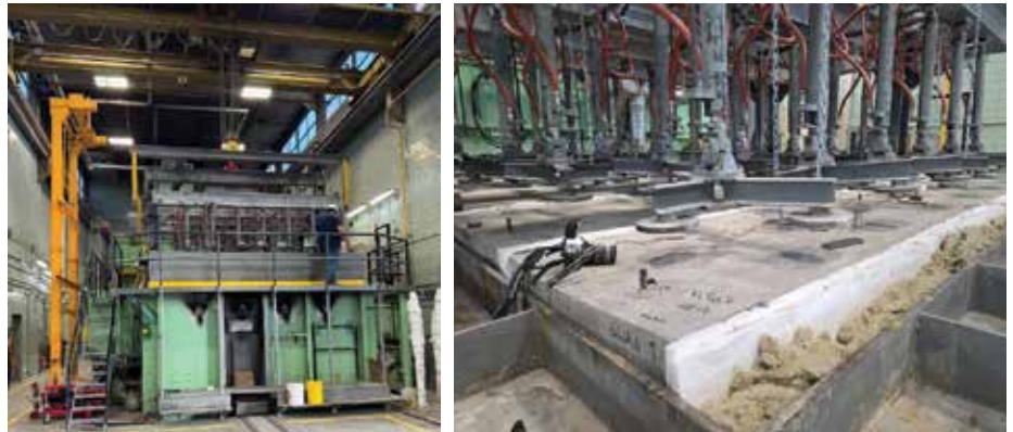
Fig. 3: Ongoing research led by Mark Green, Queen's University, and Hamzeh Hajiloo, Carleton University, on GFRP-reinforced concrete under fire (Photos courtesy of MST Rebar Inc.)
