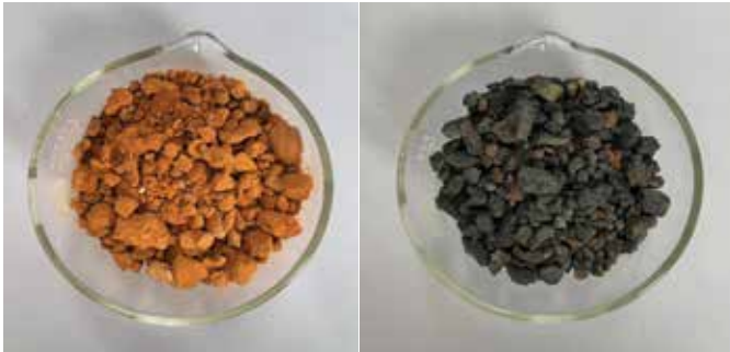
Fig. 3: Calcined clay after exiting the kiln is both reddish (left) and gray (right) in color
