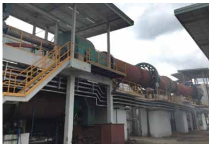
Fig. 2: Rotary kiln used to calcine clay
