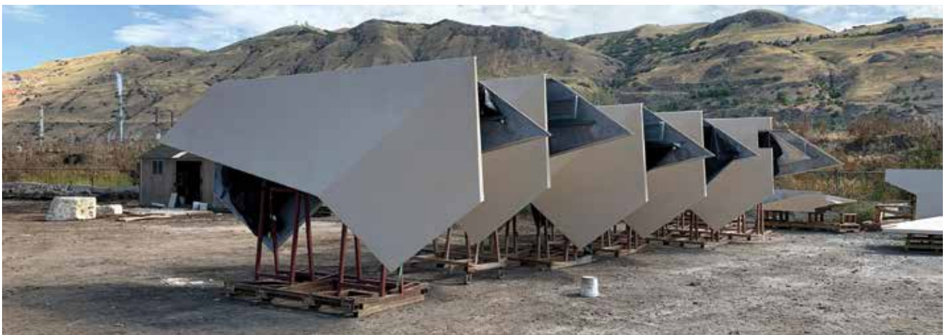
Fig. 5: Set of GFRC panels for the Walton Center manufactured by Unlimited Designs (courtesy of Unlimited Designs)
