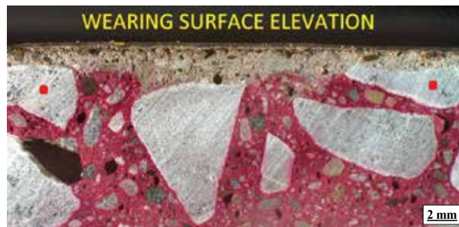
Fig. 1: A saw-cut surface of a scaled air-entrained Type IL cement and slag cement concrete core section containing a durable limestone coarse aggregate after the application of phenolphthalein. The compromised wearing surface layer (mortar) is carbonated (no pink color)
