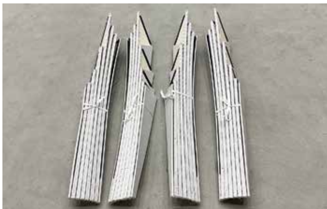
Four folded formwork sections are ready for deployment
