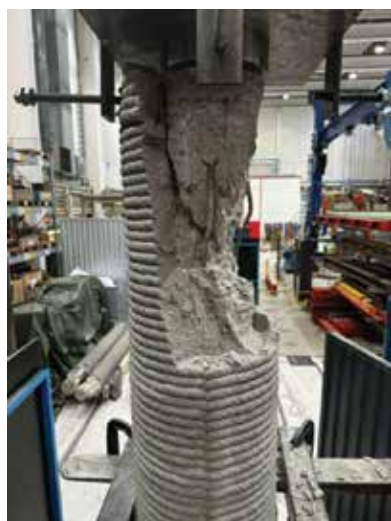
Fig. 3: Column No. III after failure
