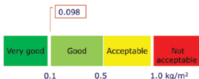
Fig. 4: Scaling mass after freezing-and-thawing tests per Swedish standard SS 137244:2019 9 classification (Note: 1 \text{ kg}/\text{m}^2 = 0.21 \text{ lb}/\text{ft}^2 )
