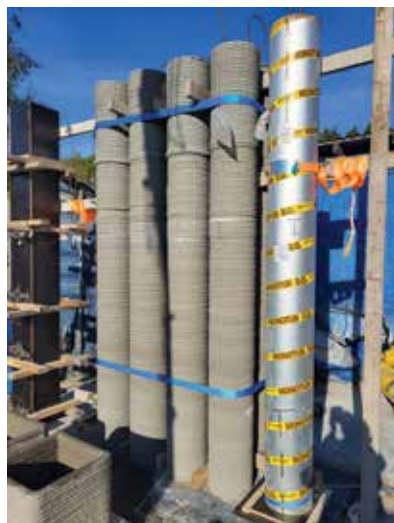
Fig. 1: 3DPC forms and a cardboard form prior to casting SCC. A rectangular 3DPC form is visible in the bottom left corner of the photo. This form was used for enabling coring of samples for subsequent durability tests
