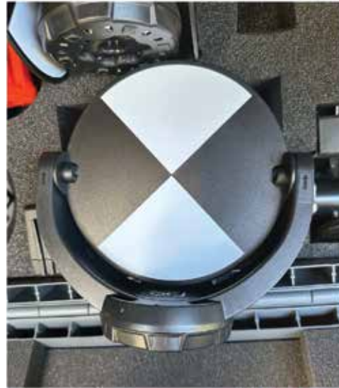
Fig. 2: One of the black and white (B/W) paper targets used during testing
