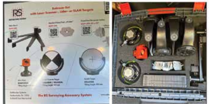
Fig. 4: The control points consisted of B/W paddle targets designed to be rotated around the center axes for line-of-sight measurements
