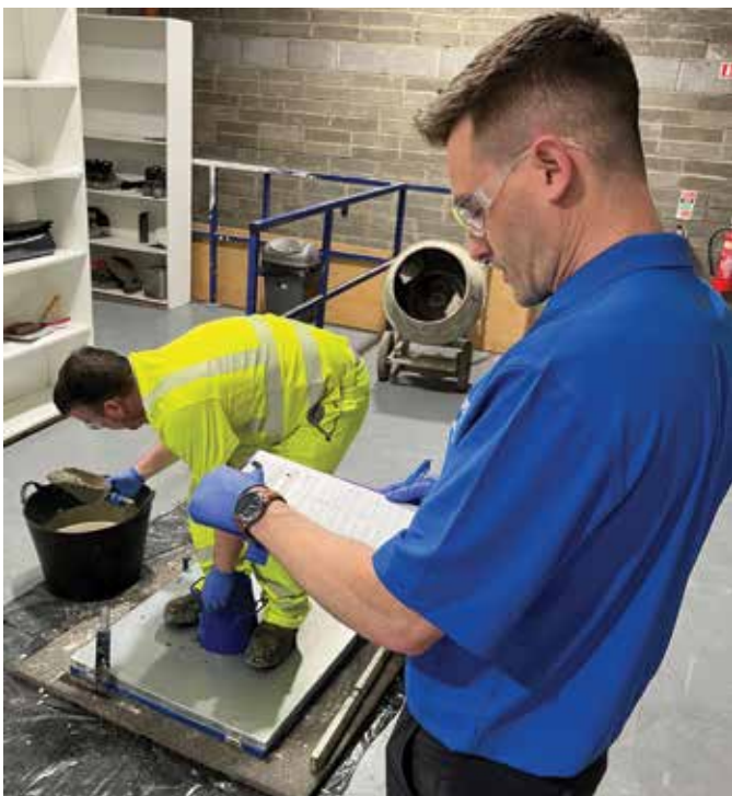
Certification examiner overseeing an EN flow table test
