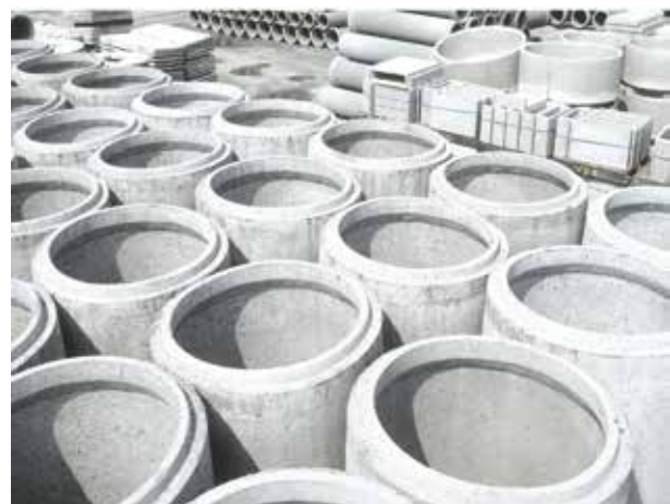
Fig. 2: Precast pipes with steel fibers have been manufactured by SIMAT in France since 1995
