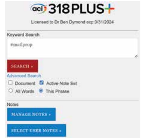
Fig. 2: Screenshot of ACI 318 PLUS navigation toolbar where users can search by keyword (#matlprop in this figure), manage notes, and select which user notes to display
