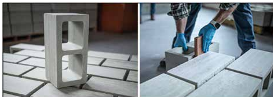
Fig. 1: Biological CMU blocks (photos courtesy of Prometheus Materials, Inc.)
