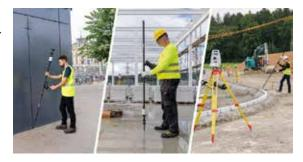
put the user at risk. By updating the pole height automatically in the field software, the system ensures that the height on record is always correct, which avoids errors, time-consuming postprocessing, and returning to the field to remeasure. Additionally, the AP20 AutoPole's target identification ensures the user's instrument will always lock to the correct target.
