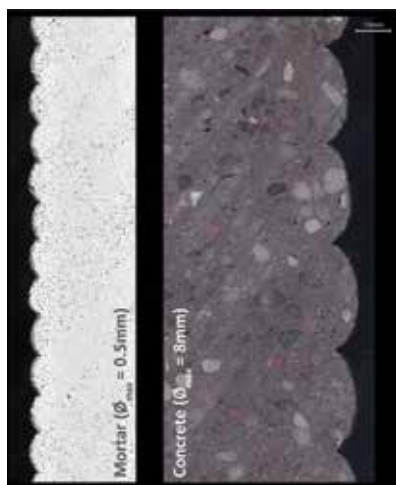
Fig. 3: Close-up view of 3DCP samples produced with mortar and concrete
