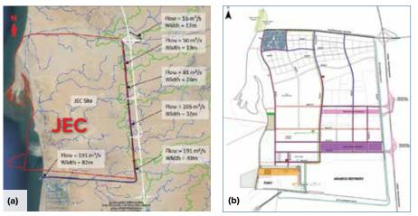
Fig. 2: JEC flood mitigation channel: (a) cumulative design flows and required widths; and (b) the channel passes the Aramco Refinery, located at the southeast corner of the site
