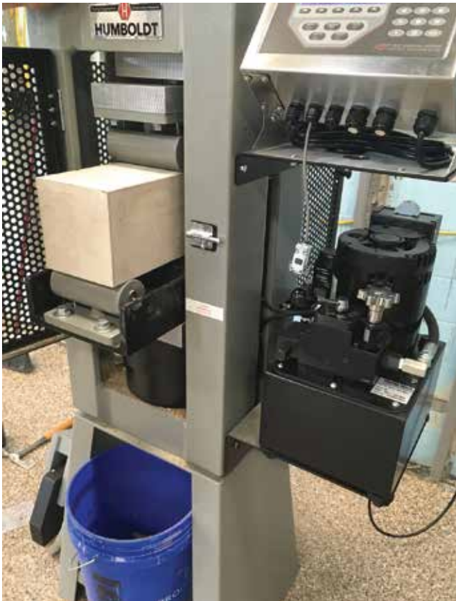
Fig. 6: Typical flexural test setup per ASTM C78/C78M
